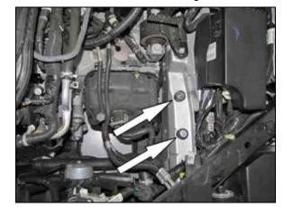
8. Install the two provided rubber mounted studs
