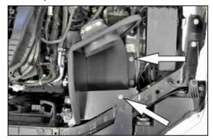
13. Install the heat shield assembly onto the rubber mounted studs and secure with the provided hardware.
