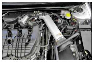
15. Install the K&N<sup>®</sup> intake tube into the silicone hose at the filter adapter and then into the hose at the intake plenum, then secure with the provided hose clamp.
