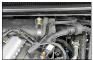
12. Install the provided silicone hose (08699) onto the intake plenum and secure with the provided hose clamp.
