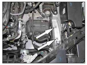
two air box mounting studs shown. 7. Remove the
