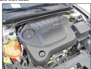
2. Lift up the engine cover and remove it from the top of the engine
