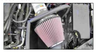
17. Install the K&N<sup>®</sup> air filter onto the filter adapter and secure with the provided hose clamp. NOTE: Drycharger<sup>®</sup> air filter wrap; part # RF-1048DK is available to purchase separately. To learn more about Drycharger<sup>®</sup> filter wraps or look up color availability please visit http://www.knfilters.com<sup>®</sup>.
