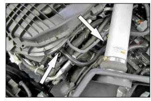
16. Install the provided crank case vent hose onto the fitting installed into the K&N<sup>®</sup> intake tube and then onto the factory fitting on the valve cover. **NOTE: It may be necessary to rotate the heater hose spring clamp so that it does not contact the crank case vent hose.**
