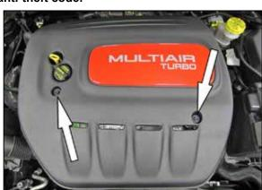
2. Remove the two bolts securing the engine cover and then remove the cover from the vehicle.
