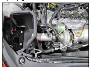
17. Connect the crank case vent hose, EVAP vent hose and BOV hose the fittings installed into the K&N® intake tube.
