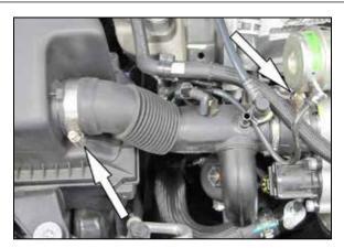
4. Loosen the hose clamps securing the intake tube to the turbo inlet and air box. Then remove the stock intake tube.
