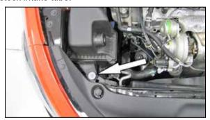
5. Remove the bolt securing the factory air box and then remove the factory air box from the vehicle.
