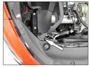
16. Secure the heat shield mounting bracket with the factory bolt removed in step #5 but do not completely tighten at this time.
