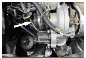
12. Install the provided silicone hose (5-222N) onto the turbo inlet and secure with the provided hose clamp.
