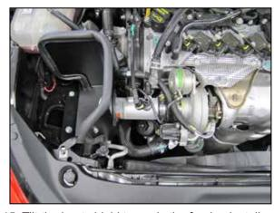
15. Tilt the heat shield towards the fender, install the K&N® intake tube through the hole in the heat shield and then install into the silicone hose on the turbo. Rotate the tube so the vent fittings align with the factory hoses and then secure the tube with the provided hose clamp.
