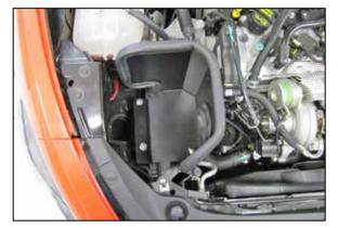
11. Install the heat shield into position so the standoffs set into the air box mounting grommets. NOTE: Do not secure the mounting bracket to the core support at this time.
