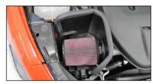
20. Install the K&N® air filter and secure with the provided hose clamp.
