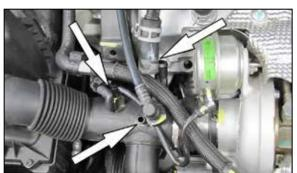
3. Disconnect the crankcase vent hose, EVAP hose and BOV valve hose from the stock intake tube as shown.
