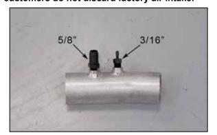
14. Install the 3/16" vent fitting and 5/8" vent fitting into the K&N® intake tube as shown. Note: NPT fitting has tapered threads and only designed to be installed until hand tight, then tighten one rotation or when the fitting becomes difficult to return.
