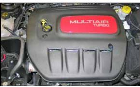
19. Reinstall the engine cover and secure with the factory mounting bolts. Adjust and heat shield for best fit and then secure with the hardware and hose clamps provided.
