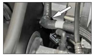
18. Remove the factory coolant hose retaining clip, then install the provided mounting head tie wrap into the lower hole in the heat shield and secure the coolant hose as shown.
