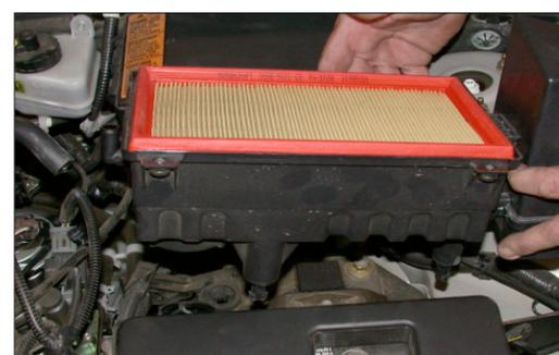
6. Pull firmly upwards to remove the lower air cleaner assembly as shown.
