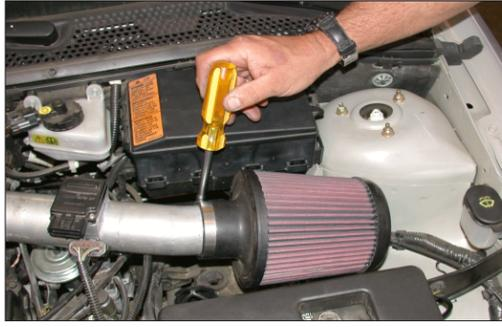
13. Install the K&N® air filter onto the K&N® Typhoon® intake tube and tighten with the provided hose clamp as shown.
