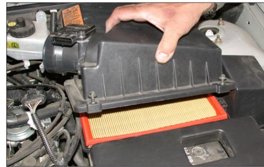
4. Remove the four bolts that secure the air cleaner cover, then remove the cover and filter as shown.
