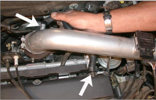
12. Using the provided vent hose, (Trim to fit), connect to the K&N® Typhoon® intake tube and valve cover as shown.
