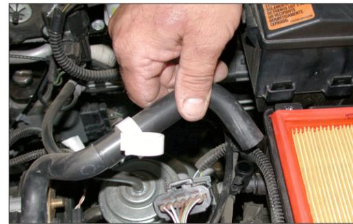
5. Remove the vent hose from the side of the lower air cleaner and valve cover.
