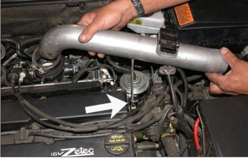
11. Install the K&N® Typhoon® intake tube into the silicone hose then line up the bracket with the ignition bracket and secure with the bolt from step 10. Tighten the hose clamps using the 9/64 allen wrench provided.
