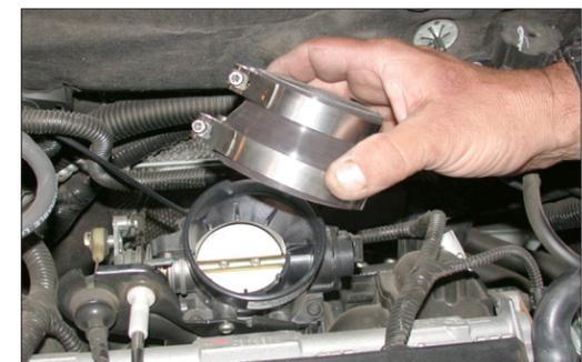
7. Install the provided silicone hose and hose clamps onto the throttle body as shown.
