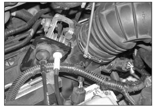
6. Remove the clamp at the throttle body as shown.
