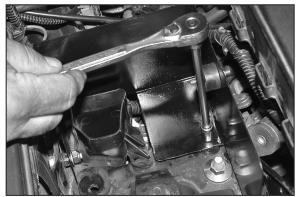
13. Secure the heat shield to the rubber mounted stud using the provided hardware as shown.
