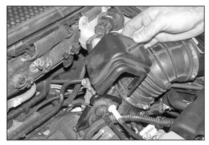
3. Pull up firmly to remove the plastic throttle linkage cover as shown.
