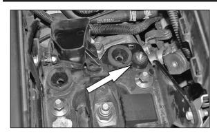
10. Install the rubber mounted stud onto the battery tray and secure with the provided hardware as shown.
