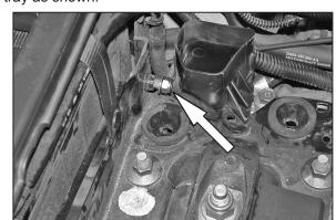
9. Install the provided nut and washer onto the stock bolt on the air cleaner tray as shown.
