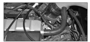
23. Reconnect the crank case vent hose to the cam cover as shown.
