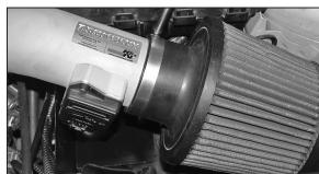
21. Install the air filter onto the Typhoon® intake tube and tighten as shown.
