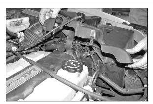
4. Pull up firmly to remove the plastic coil cover as
