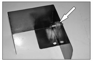
11. Install the rubber mounted stud onto the heat shield and secure it with the provided hardware as shown.
