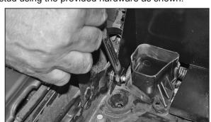
14. Tighten the hex nut on the heat shield as shown.
