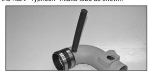
17. Install the provided silicone hose onto the vent on the K&N® Typhoon® intake tube as shown.
