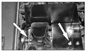
12. Install the heat shield into the vehicle and slide the slot on the heat shield onto the bolt from step 9, then, line up the hole with the rubber mounted stud from step 10 as shown.
