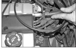
5. Disconnect the crank case vent hose from the cam cover as shown.
