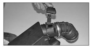
15. Remove the mass air sensor from the stock air cleaner assembly as shown using the provided Torx wrench.
