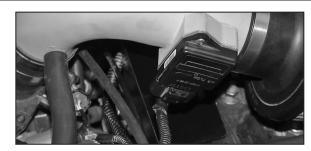
24. Reconnect the mass air sensor electrical connection as shown.
