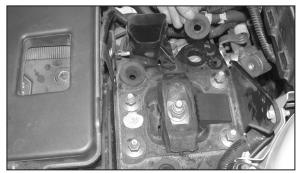
8. Remove the rubber bumper from the air cleaner tray as shown.
