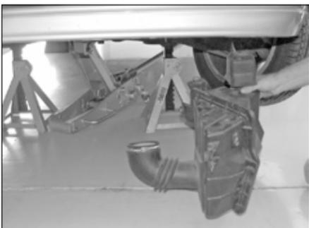
14. Lower and remove the air box assembly from the vehicle.
