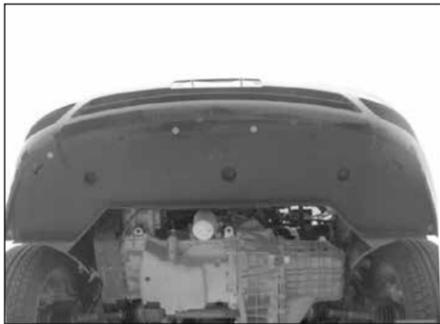
27. On vehicle's that were equipped with the splash shield, reinstall with the bolts removed in step #10a.
