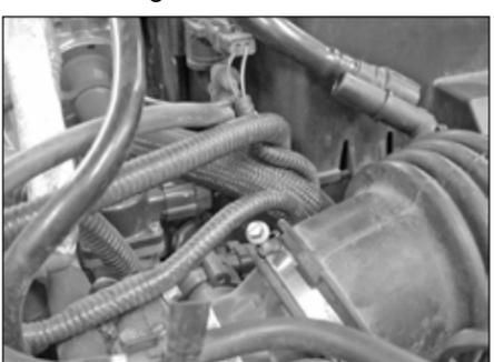
3. Loosen the hose clamp, which secures the factory intake tube to the throttle body.
