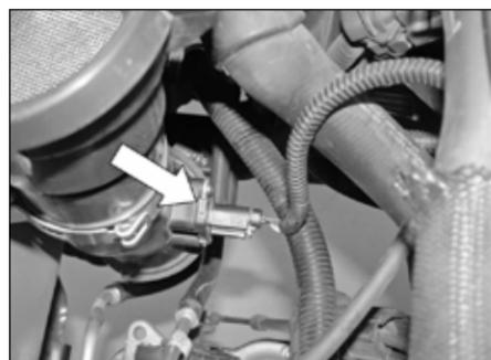
6. Depress the locking tab on the mass air sensor electrical connection and then disconnect the electrical connection.
