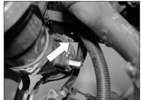
7. Loosen the hose clamp, which secures the mass air sensor housing to the lower intake housing.
