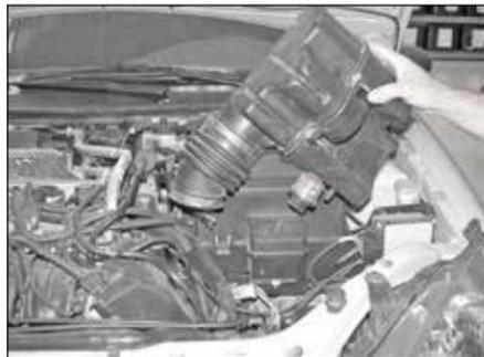
5. Lift firmly to separate the upper intake housing from the mass air sensor housing and then remove the upper intake housing from the vehicle.
