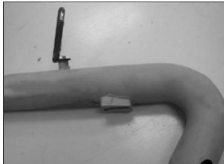
17. Install the supplied "L" bracket and hardware to the K&N® intake kit. Do not tighten completely. **NOTE: Before installing the "L" bracket, inspect the inside of the tube for any debris, then clean the inside out with water and a towel. Inspect the tube one more time before proceeding to the next step.**
