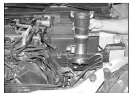
9. Pull firmly up and remove the mass air sensor assembly from the vehicle.
