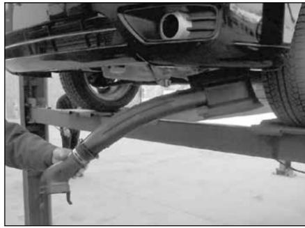
14a. On vehicle's equipped with the upper intake snorkel, pull down on the snorkel to dislodge it from the mount and then remove it from behind the fender.
