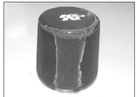
24. Install the K&N® Drycharger® onto the K&N® air filter as shown.
