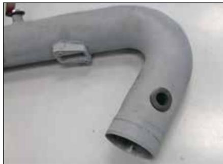
18. Install the supplied rubber grommet into the intake tube as shown.
