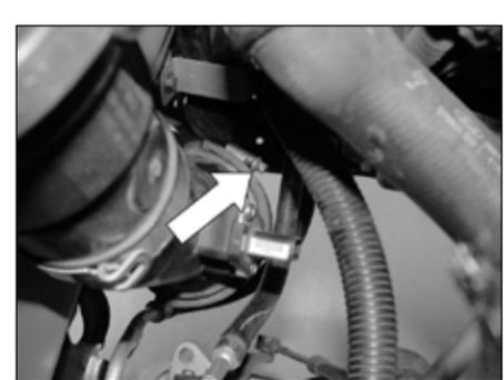
7. Loosen the hose clamp, which secures the mass air sensor housing to the lower intake housing.
