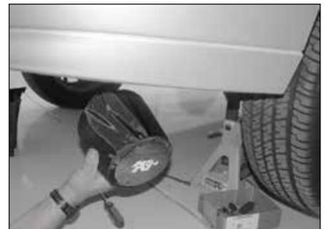
25. From underneath the vehicle, install the K&N® air filter onto the intake tube and tighten hose clamp completely.
