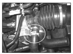
3. On vehicles equipped with an air injection pump, using pliers, release the spring clamp that fastens the air injection hose to the factory intake tube. Disconnect the air injection hose from the intake
