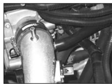
21. Connect the crank case vent hose to the  $K\&N^{\circledR}$  intake tube.
