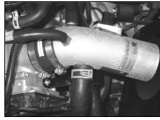
23. Connect the stock air injection hose to the fitting on the  $K\&N^{\textcircled{R}}$  intake tube, then fasten using the stock spring clamp.
