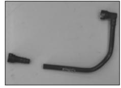
12. Disconnect the crank case vent hose from the valve cover and remove it. Place it on a surface suitable for cutting. Using a a razor blade or knife, cut the crank case vent hose as shown.
