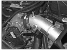
20. Install the K&N<sup>®</sup> intake tube into the silicone hose (08440) and align the tube mounting bracket (06491) with the intake tube fastening location. Secure the intake tube hose clamps and mounting bracket hardware.
