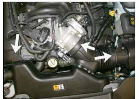
6. Loosen the hose clamps at the throttle body and the factory air box, and then remove the intake tube retaining nut shown.
