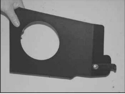
11. Install the "L" bracket (07158) onto the front of the heat shield as shown with the provided hardware.
