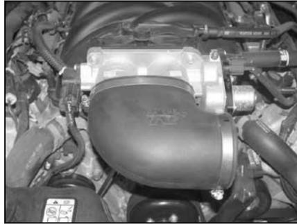
18. Install the silicone hose (084094) onto the throttle body with the provided hose clamp as shown.
