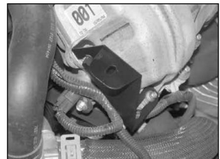
9. Install the tube-mounting bracket onto the valve cover as shown and secure with the stock hardware removed in step #7.
