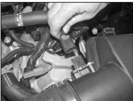
2. Release the red locking tab and then disconnect the mass air sensor electrical connection
