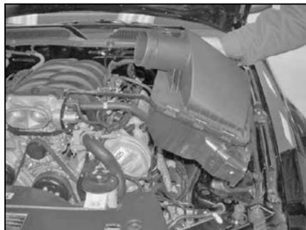
6. Remove the air box assembly as shown. **NOTE: K&N recommends customers do not discard their factory air intake.**
