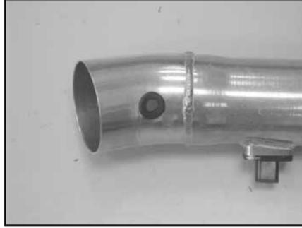
17. Install the grommet provided into the K&N® intake tube as shown.
