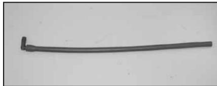
20. Install the provided 90 deg hose mender into the provided crankcase vent hose as shown.
