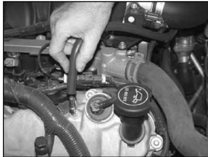
21. Install the crank case vent hose mender into the grommet installed in the K&N® intake tube and then onto the valve cover as shown.
