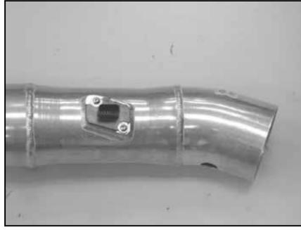
16. Install the mass air sensor into the K&N® intake tube with the provided hardware as shown.
