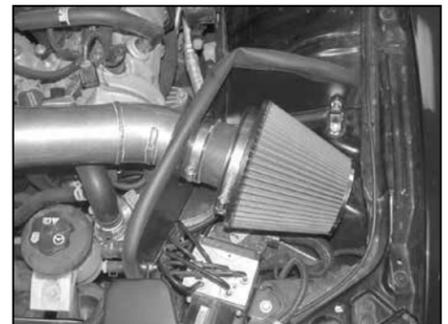
26. Install the air filter assembly onto the K&N® intake tube as shown and secure with the provided hose clamp.
