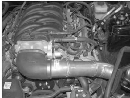
19. Install the K&N® intake tube into the silicone hose at the throttle body and onto the mounting bracket installed in step #9, then secure with provided hose clamp and 6mm bolt.
