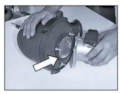
12. Remove the mass air sensor from the air cleaner.
