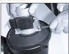
11. Loosen and remove the 4 nuts that retain the mass air sensor.
