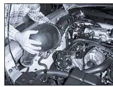
8. Remove the entire air intake assembly.
