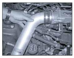
24. Install the complete  $K\&N^{\otimes}$  intake assembly into the vehicle and slide the tube into the silicone hose on the throttle body as shown.
