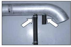
19. Install the provided hoses from the previous step onto the  $K\&N^{\circledast}$  intake tube and secure with the provided hose clamps as shown.
