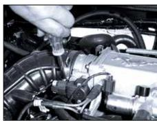
4. Loosen the hose clamp on the intake tube at the throttle body.
