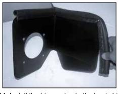
14. Install the trim seal onto the heat shield. NOTE: Some cutting and trimming will be necessary to achieve best fit.
