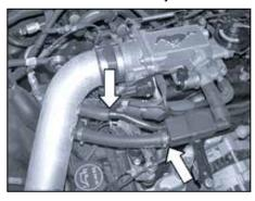
26. Reconnect the vent hoses to the K&N $^{\circ}$  intake tube as shown and tighten hose clamps.
