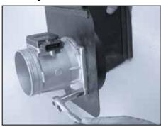
15. Assemble the mass air sensor, heat shield and adapter, using the gaskets and hardware provided as shown, but do not tighten completely at this time.
