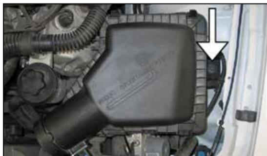
6. Remove the bolt shown that secures the factory airbox to the fender well.
