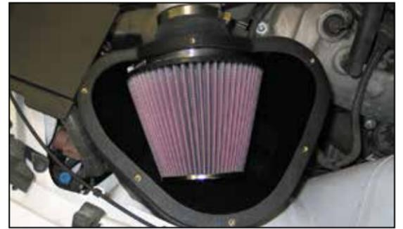
24. Install the K&N® air filter onto the filter adapter and secure with the provided hose clamp.
