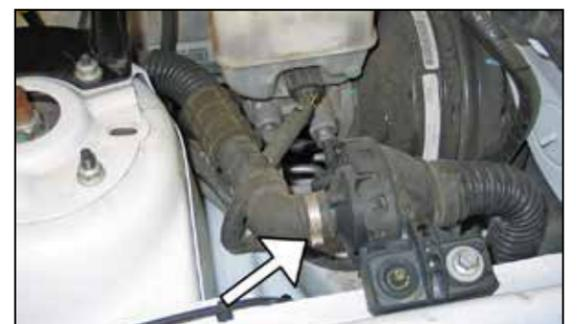
8. Cut the hose clamp securing the engine pulse hose to the engine pulse drum.
