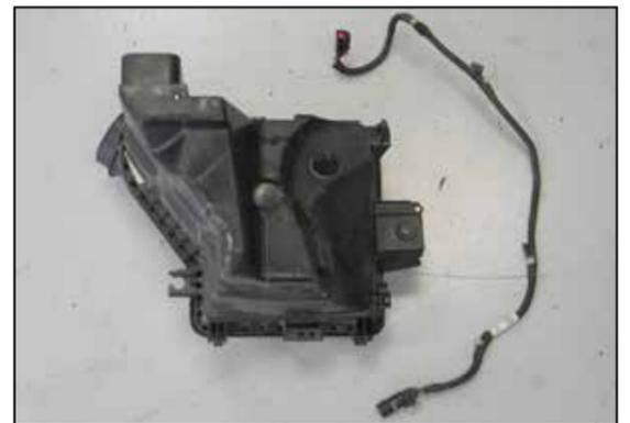
26. Remove the mass air sensor wiring harness from the factory airbox.
