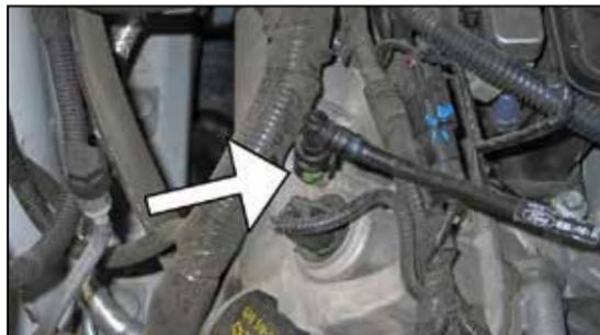
4. Release the locking tab and then disconnect the crankcase vent tube from the valve cover.
