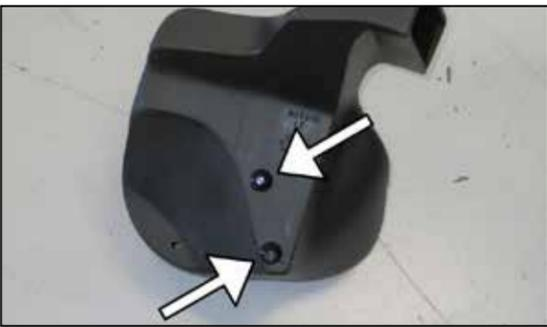
12. Install the two provided mounting studs onto the bottom of the K&N® airbox using the provided hardware.
