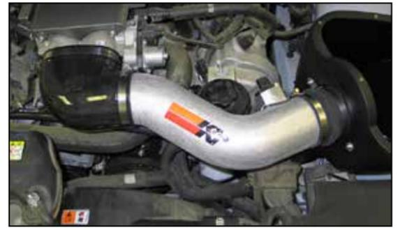
22. Install the K&N® intake tube assembly into the silicone hose on the filter adapter, and then into the 90° hose attached to the throttle body. Adjust the tube and hose for proper fit, then tighten the hose clamps.
