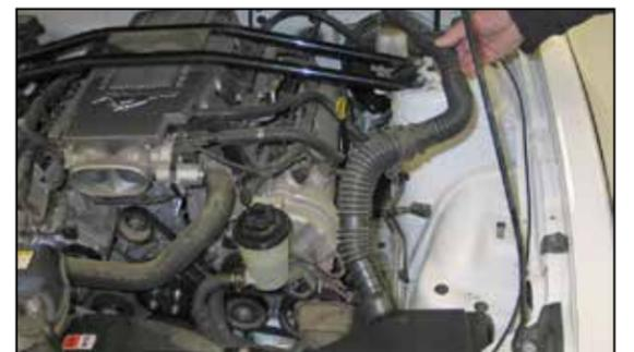
9. Remove the engine pulse hose from the vehicle.
