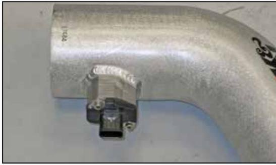
17. Install the mass air sensor into the K&N® intake tube and secure with the provided hardware.
