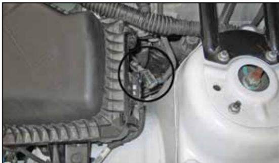
2. Disconnect the mass air sensor harness electrical connection at the rear of the airbox.
