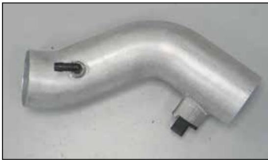
18. Install the 90° vent fitting into the K&N® intake tube as shown.
