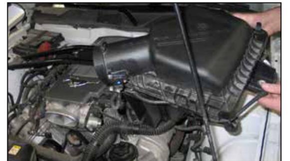
7. Remove the factory airbox from the vehicle. **NOTE: K&N Engineering, Inc., recommends that customers do not discard factory air intake.**
