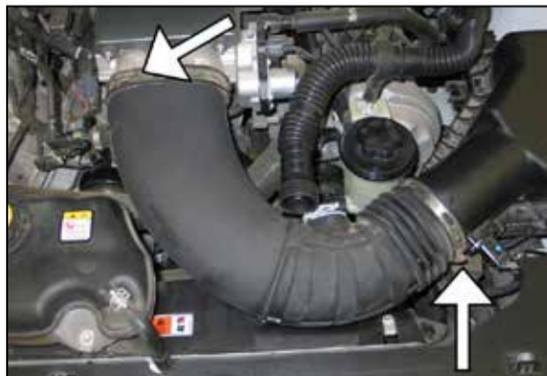
5. Loosen the two hose clamps that secure the intake tube to the throttle body and airbox, and then remove the intake tube from the vehicle.
