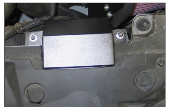
23. Install the fresh air intake scoop into position and secure to the heat shield and core support with the provided hardware.
