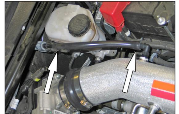
21. Connect the provided EVAP hose onto the 90° vent fitting installed in the K&N® intake tube, then connect the open end to the EVAP check valve as shown.
