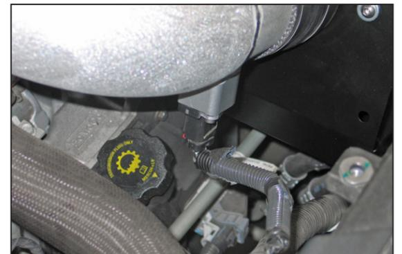
22. Reconnect the mass air sensor electrical connection.
