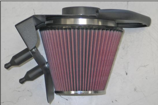
12. Install the K&N® air filter onto the filter adapter and secure with the provided hose clamp.
