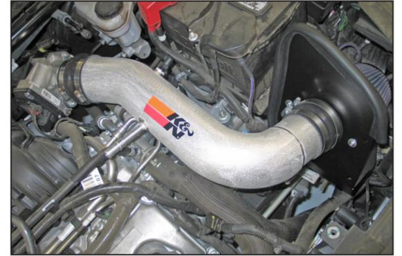
19. Install the K&N® intake tube assembly into the hose at the throttle body and then onto the filter adapter and secure with the provided hose clamp.
