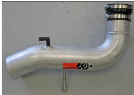
18. Install the provided silicone hose (084091) onto the K&N® intake tube as shown and secure with the provided hose clamp.
