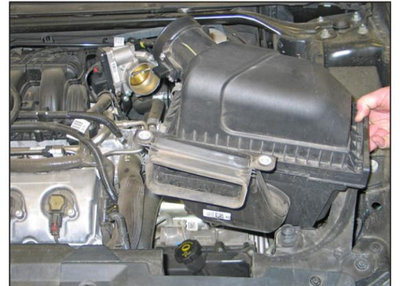
8. Lift up the airbox assembly to dislodge it from the mounting grommets and then remove the airbox from the vehicle.
