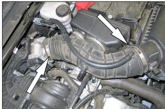
5. Loosen the two hose clamps that secure the stock intake tube to the throttle body and air filter housing.
