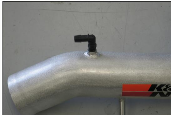
16. Install the provided 90° NPT vent fitting into the K&N® intake tube as shown.
