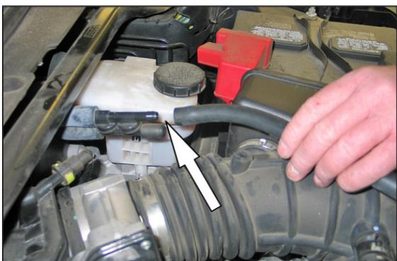
3. Disconnect the EVAP hose from the check valve connection.
