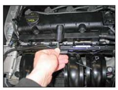
21a. Remove the rubber hose from the crankcase vent assembly and attach it to the valve cover as shown. Install the  $\frac{1}{4}$ " 90° vent into the rubber hose as shown.'
