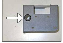
11. Install the provided grommet into the bottom of the heat shield as shown.
