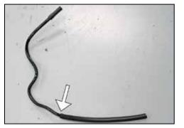
21. US Models Only: Install the provided 1/2" silicone vent hose onto the cut vent tube as shown. 24. Install the fresh air scoop into the scoop attached to the heat shield and then reattach to the factory connection on the core support.
