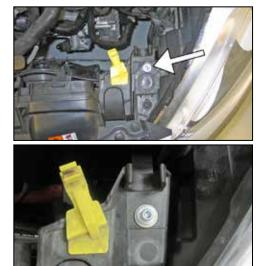
9. Install the provided 30mm long Allen bolt and washer into the air box mounting bracket hole as shown. On some models it may be necessary to use the supplied larger washer.
