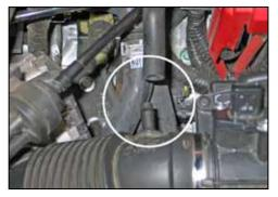
3. When equipped with EVAP, disconnect the EVAP vent line from the factory intake tube as shown.
