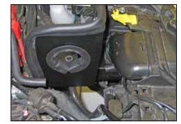
14. Install the 10" section of edge trim into the hole of the heat shield as shown.
