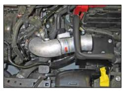
29. When equipped with EVAP, install the K&N<sup>®</sup> intake tube into the silicone hose at the throttle body and secure with the provided hose clamp. Attach the crankcase vent hose to the installed npt vent fitting.
