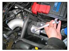
28a. Models without EVAP: Pass the K&N<sup>®</sup> intake tube through the heat shield and rotate so the provided NPT plug (08032) can be installed into the K&N<sup>®</sup> intake tube as shown.
