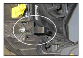
10. Install the heat shield mounting bracket (07195) onto the bottom of the bolt installed in the previous step along with the spacer provided.
