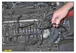
5. Release the locking collar for the crankcase vent hose to the airbox connection by pulling it back, so the crankcase vent hose can be disconnected from
