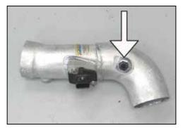
27. Install the provided 3/8"NPT vent fitting into the K&N<sup>®</sup> intake tube as shown. NOTE: Plastic NPT fittings are easy to cross thread. Install the vent fitting "hand" tight, then turn it two complete turns with a wrench.
