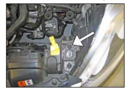
the mass air sensor electrical connection.
