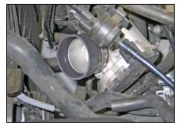
19. Install the provided silicone hose (08476) onto the throttle body and secure with the provided hose clamp.
