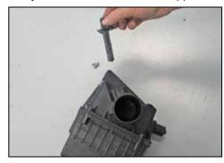
25. Remove the two bolts securing the mass air sensor to the factory airbox and then remove the mass air sensor from the airbox. NOTE: Some vehicles may not be equipped with a mass air sensor.
