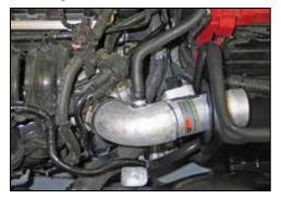
30. When equipped with EVAP, install the EVAP vent hose to the npt vent fitting. NOTE: Models without EVAP, attach the crankcase vent hose to the NPT vent fitting.
