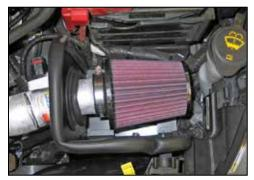
32. Install the K&N<sup>®</sup> air filter and secure with the provided hose clamp.
