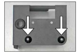
12. Install the two provided heat shield mounting studs to the bottom of the heat shield as shown using the provided hardware.
