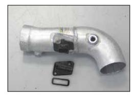
26. On vehicles that are equipped with a mass air sensor install the sensor into the K&N<sup>®</sup> intake tube and secure with the provided hardware. On all other vehicles, install the provided gasket onto the block off plate and install the block off plate into the K&N<sup>®</sup> intake tube and secure with the provided hardware.
