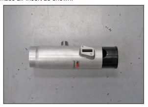
11. Install the mass air insert into the K&N<sup>®</sup> intake tube so that the hole in the insert aligns with the mass air location in the tube.
