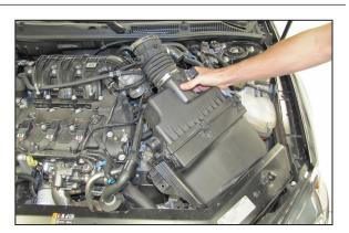
7. Lift up and remove the complete intake system as shown.
