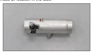
12. Install the mass air sensor and secure with the provided hardware.
