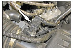
4. Release the red locking tab and then disconnect the mass air sensor electrical connection.
