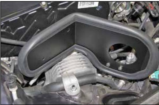
9. Install the heat shield onto the mounting bracket and secure with the provided hardware and spacers, the spacers are to be placed between the bracket and heat shield.
