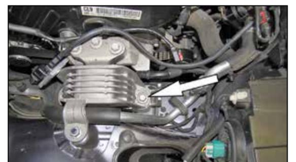
6. Remove the motor mount bolt show.
