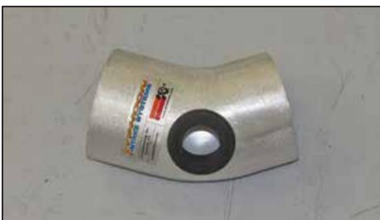
12. Install the provided grommet into the K&N® intake tube as shown.
