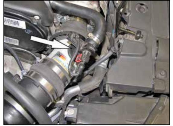
19. Connect the Pressure sensor to the quick disconnect fitting installed into the K&N® intake tube.
