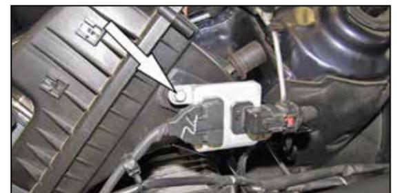
5. Lift up the air filter assembly to gain access to the electrical box attached to the air filter housing. Remove the two bolts that secure the electrical box and separate it from the air filter housing and then remove the air filter assembly from the vehicle. **NOTE: The air box has a drain tube attached that will need to be separated before the housing is removed.** **NOTE: K&N Engineering, Inc., recommends that customers do not discard factory air intake.**
