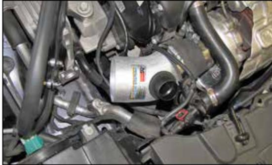
14. Install the K&N® intake tube into the coupler at the turbo but do not completely tighten at this time.
