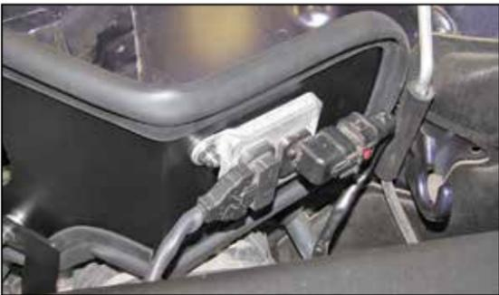
10. Using the provided hardware, secure the electrical box to the heat shield as shown.
