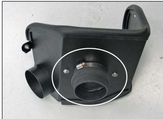
14. Install the silicone hump hose (08699) onto the filter adapter as shown, secure with the provided hose clamp.
