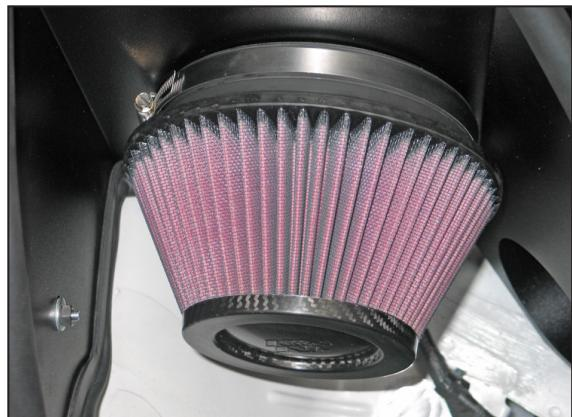
18. Install the K&N® air filter and secure with the provided hose clamp.
