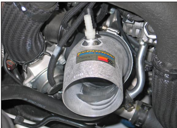
9. Install the K&N® intake tube into the silicone hose and secure with the provided hose clamp.
