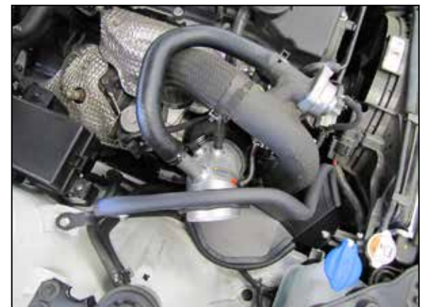
19. Connect the BOV and EVAP hoses to the K&N® intake tube.
