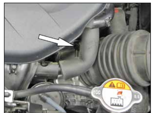
5. Loosen the hose clamp securing intake tube to the throttle body.
