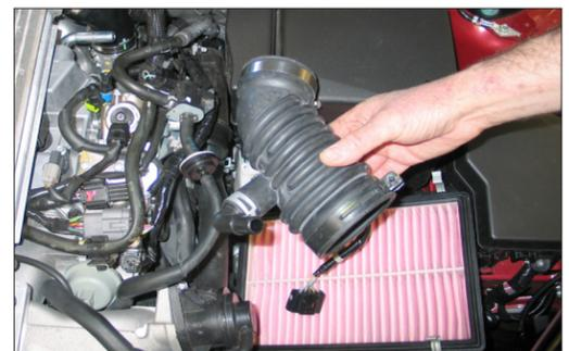
8. Remove the intake tube from the vehicle.
