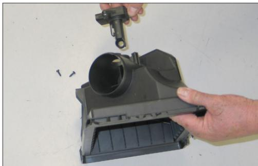
19. Remove the screws securing the mass air sensor and then remove the mass air sensor from the upper air box.
