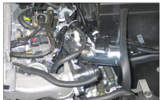
24. Install the K&N® intake tube assembly into the silicone hose at the turbo inlet pipe and align the bracket with the pop off valve mounting location. Secure the intake tube with the provided hose clamp and hardware.
