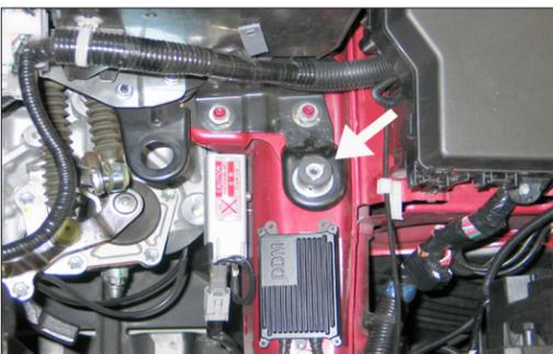
15. Install the provided rubber mounted stud onto the air box mounting bracket as shown using the provided hardware.
