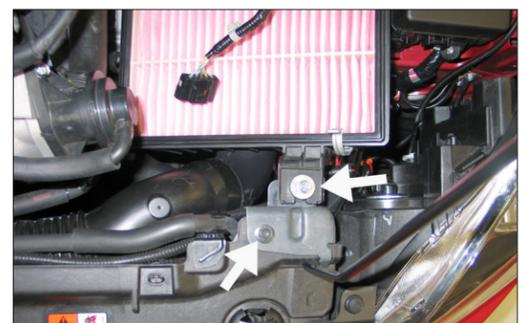
9. Remove the two bolts shown and then remove the front air box mounting bracket from the vehicle. **NOTE: The bolt which secures the bracket to the core support will be reused in a later step.**
