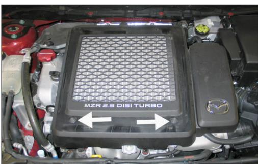
3. Remove the two bolts that secure the engine cover and then remove the engine cover from the vehicle.
