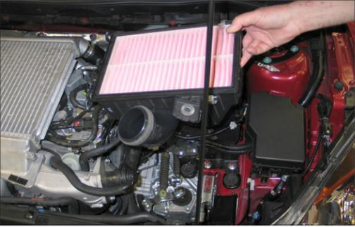
11. Remove the lower air box from the vehicle.
