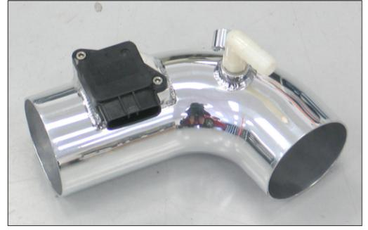
21. Install provided 90° npt fitting into the K&N® intake tube as shown.
