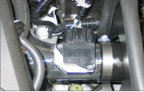
28. Reconnect the mass air sensor electrical connection.
