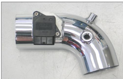
20. Install the mass air sensor into the K&N® intake tube and secure with the provided hardware.
