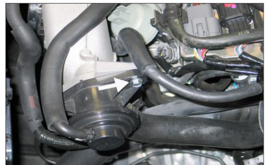
23. Remove the pop off valve upper mounting bolt shown.
