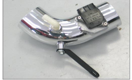
22. Install the tube mounting bracket (083130) onto the K&N® intake tube as shown.
