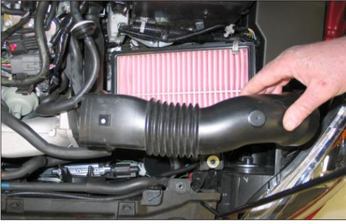
10. Unhook the fresh air duct from the air box and then remove it from the vehicle.
