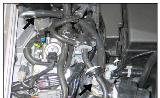
25. Install the provided crank case vent hose onto the 90° fitting in the K&N® intake tube and then attach the open end to the valve cover port.
