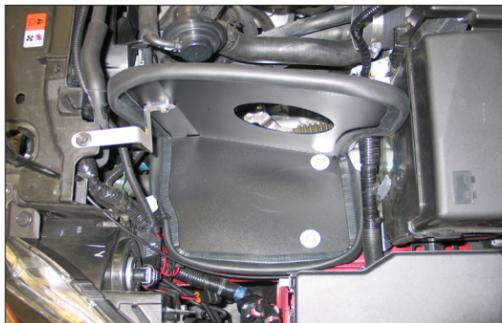
18. Install the heat shield into position on the air box mounting bracket then secure the heat shield with the provided hardware.
