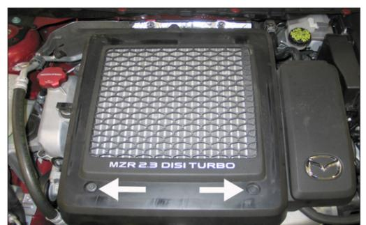
26. Reinstall the engine cover and secure with the factory bolts.
