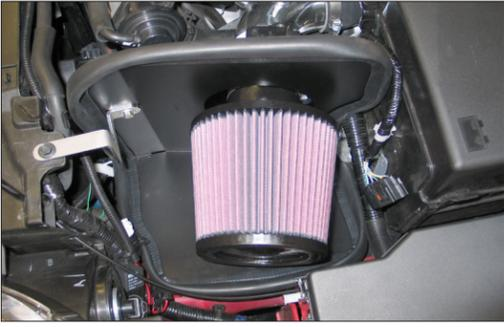
27. Install the K&N® air filter onto the intake tube and secure with the provided hose clamp.
