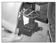
14. From underneath the vehicle loosen and remove the three nuts that secure the air intake resonator, then remove the resonator as shown.
