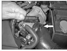
3. On 2004 and earlier models, disconnect the stock crank case vent from the stock intake tube.
