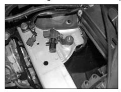
22. Secure the solenoid/bracket assembly to the threaded hole from step 21 using the provided rubber molunted stud.
