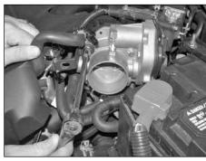
18. Install the provided "Z" bracket onto the throttle body using the stock bolt
