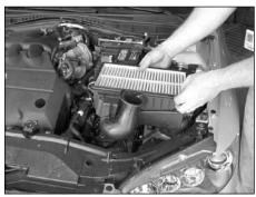
10. Pull firmly upwards to release the lower air cleaner assembly from the factory grommets.
