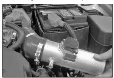
33. Install the hose clamp onto the silicone hose, then slide the short ram intake tube into the silicone hose. Do not tighten at this time.
