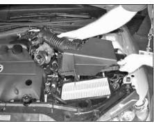
7. Unclip the air cleaner lid; then, remove the upper air cleaner assembly.
