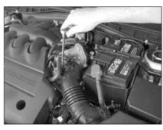
6. Loosen the hose clamp at the throttle body.
