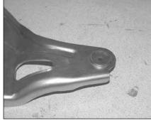
24. Insert the provided rubber washer into the hole on the stock support bracket as shown.
