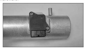
32. Install the stock mass air sensor into the adapter on the K&N® Typhoon® short ram tube and secure with the provided hardware.
