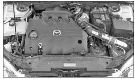
47. Reconnect the vehicle's negative battery cable. Double check to make sure everything is tight and properly positioned before starting the vehicle.
