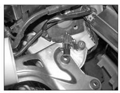
37. Reconnect the solenoid electrical connection as shown.
