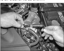
17. On 2004 and earlier models, remove the  $90^{\circ}$  vent fitting and rubber hose from the crank case vent hard line.
