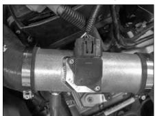
46. Reconnect the mass air sensor electrical connection as shown.
