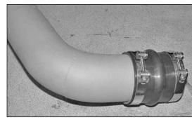
38. Slide the silicone hump hose and hose clamps onto the K&N® cold air tube as shown.
