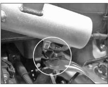
34. Secure the short ram intake tube to the "Z" bracket using the provided hardware as shown in the photograph.
