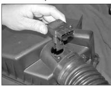
16. Remove the two screws that secure the mass air sensor, then, remove the mass air sensor from the air cleaner lid as shown.
