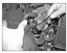
19. Secure the solenoid to the "Z" bracket using the nut removed in step 4.
