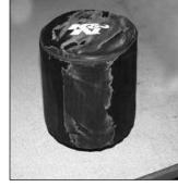
42. Install the K&N® Drycharger® onto the K&N® air filter as shown.
