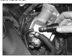
17a. On 2005 and later models, cut the crank case vent hard line just behind the "quick disconnect" fitting.
