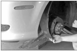
13. Remove the screws and plastic rivets, then lower the inner fender valance as shown.
