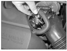
5. On 2004 and earlier models, remove the solenoid from the stock intake tube as shown.
