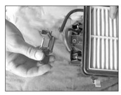
15. Disconnect the vacuum hoses from the solenoid, then remove the solenoid from the side of the air cleaner assembly as shown.
