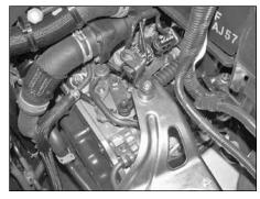
31. Install the provided "Z" bracket onto the rubber mounted stud and secure with the provided hardware.
