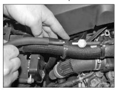
28. Remove the vacuum hose from the one way check valve as shown.
