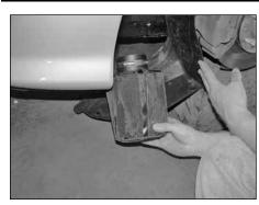
43. From underneath the vehicle install the K&N® air filter onto the cold air tube and secure with the provided hose clamp as shown.
