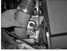
40. Secure the bracket to the rubber mounted stud using the provided hardware as shown.
