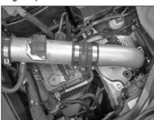
41. Slide the silicone hump hose onto the short ram tube and tighten the hose clamps.
