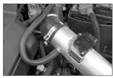
36. Connect the crank case vent hose to the vent fitting on the K&N<sup>®</sup> intake tube as shown in the photograph.
