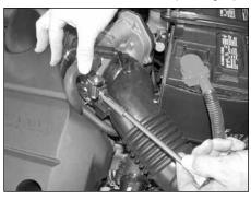
4. On 2004 and earlier models, loosen and remove the nut that secures the solenoid to the stock intake tube as shown.
