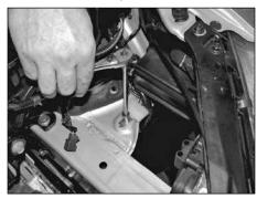
20. Remove the bolt that secures the ground block to the inner fender as shown.
