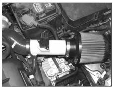
48. This K&N® Typhoon® kit has been designed to be used in two different configurations. In the case of inclement weather, the cold air tube can be removed and the air filter can be clamped onto the intake tube located in the engine compartment to avoid the possibility of ingesting water into the engine.
