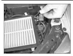
9. Disconnect the solenoid electrical connection on the side of the lower air cleaner assembly as shown.
