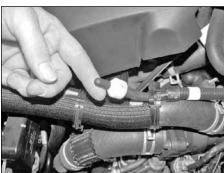
29. Install the provided rubber cap onto the check valve as shown.
