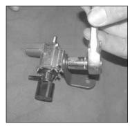
21. Secure the solenoid from step 15 to the provided "L" bracket using the nut removed in step 15.
