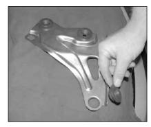
23. Remove the stock rubber grommet from the stock air cleaner support bracket as shown.
