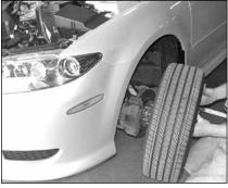
12. Lift the vehicle and support it with jack stands, then remove the front driver side tire as shown.
