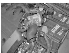
30. Install the silicone hose and hose clamp onto the throttle body as shown.
