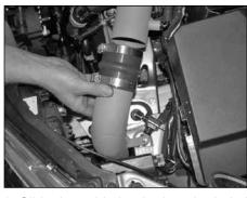
39. Slide the cold air tube into the hole in the inner fender. Then line up the tube bracket with the rubber mounted stud as shown.
