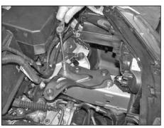
27. Secure the support bracket to the original threaded holes from step 11.
