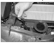
8. Disconnect the vacuum hose from the lower air cleaner assembly as shown.
