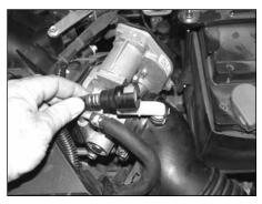
3a. On 2005 and later models, release the "quick disconnect" connector from the fitting in the stock intake tube as shown in the photograph.
