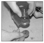
25. Secure the rubber mounted stud to the support bracket using the provided fender washers and nylock nut as shown.
