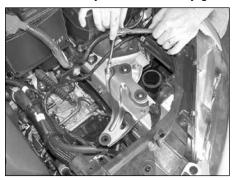
11. Loosen and remove the two bolts that secure the air cleaner support bracket to the inner fender as shown.
