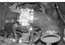
14. Install the 90 degree silicone hose onto the throttle body as shown.
