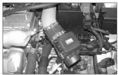
17. Slide the mass air sensor assembly onto the Typhoon intake tube as shown.
