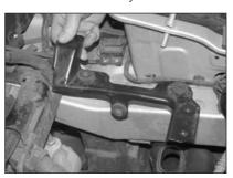
8. Loosen and remove the two bolts that secure the air cleaner support bracket, then, remove the air cleaner support bracket as shown.
