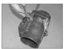
12. Using the provided hardware, secure the provided mass air adapter and the wire harness bracket to the stock mass air sensor as shown. **NOTE**: Be sure to use the stock mass air sensor gasket.
