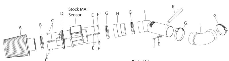
Prior to the installation process, please inspect the contents of this package to ensure that all parts are included in this kit. Please see parts list for description and quantities.
