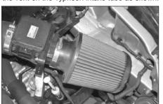
19. Install the K&N Filtercharger onto the mass air adapter and secure with the provided hose clamp.
