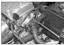
10. Remove the bolt that secures the wire harness to the engine as shown.
