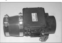
13. Install the silicone step hose and hose clamps onto the mass air sensor as shown.
