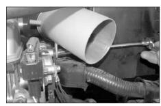
16. Using the provided hardware secure the tube bracket to the threaded boss from step 8 as shown.
