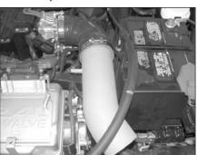
15. Install the Typhoon intake tube into the silicone hose as shown. **NOTE**: Before installing the intake tube into the silicone hose, inspect the inside of the tube for any debris, then clean the inside out with water and a towel. Inspect the tube one more time before proceeding to the next step.
