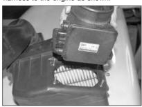
11. Remove the four nuts that secure the mass air sensor, then, remove the mass air sensor as shown.
