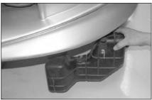
9. From underneath the vehicle remove the lower valance and loosen the three bolts that secure the air intake resonator to the inner fender, then, remove the air intake resonator from underneath the vehicle as shown.
