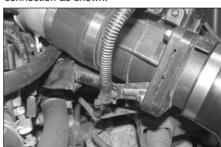
21. Re-clip the mass air sensor wire harness to the stock bracket on the mass air sensor as shown.
