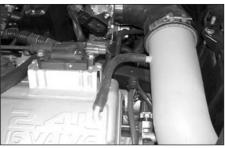
18. Install the provided silicone hose onto the vent on the cam cover, then, slide the other end onto the vent on the Typhoon intake tube as shown.
