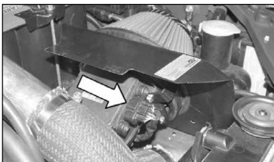
47. Reconnect the mass air sensor electrical connection as shown.
