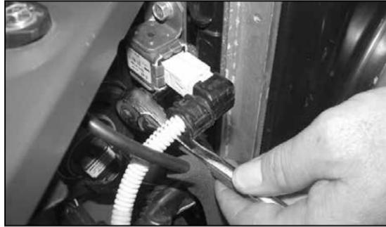
18. Remove the lower bolt that secures the air bag sensor to the radiator core support as shown. (Except UK)
