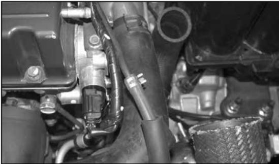
30. Reconnect the bypass valve vent hose to the hardline as shown.
