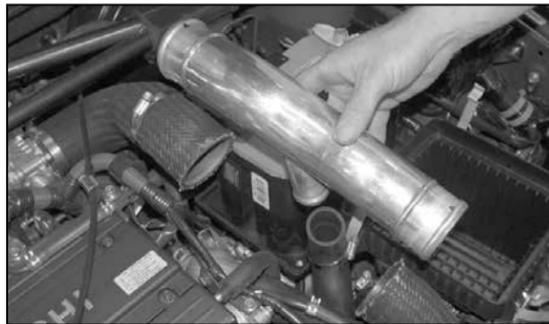
5. Pull firmly on the hoses to remove the intercooler tube as shown.
