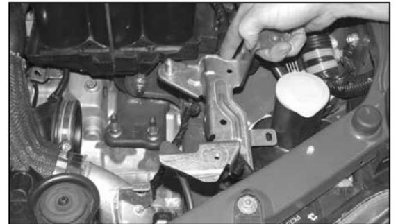
9. Lift up the air cleaner support bracket and unclip the wire harnesses, then, remove the bracket as shown.
