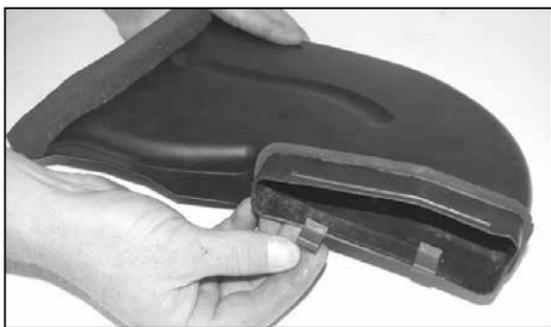
48. Install the provided retaining clips onto the stock air inlet duct as shown.
