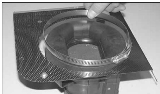
36. Slide the provided hose clamp over and onto the mass air adapter as shown.
