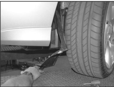
13. Remove the one screw and four push clips on the inner fender valve, then pull the valve down as shown.
