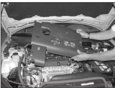
2. Remove the four bolts that secure the engine cover, then remove the engine cover as shown.
