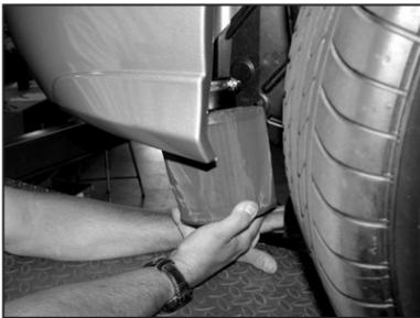
32. From underneath the vehicle install the K&N® air filter onto the cold air tube and secure with the provided hose clamp as shown.
