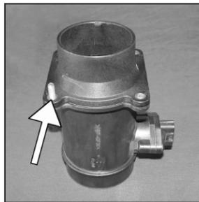
19. Secure the provided mass air adapter to the stock mass air sensor using the provided button head screws.
