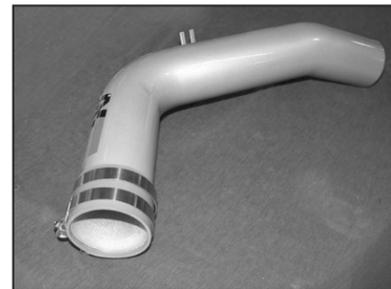
25. Install the silicone hose and hose clamps onto the K&N cold air tube as shown.
