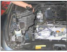
35. Remove the passenger side airbox assembly from the vehicle as shown.
