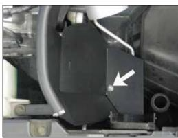
27. Install the heat shield assembly into the engine bay as shown. Secure the upper heat shield mounting bracket to the coolant reservoir using the factory bolt removed in step #11. Using the supplied hardware, secure the heat shield to the lower mounting bracket installed during step #24. NOTE: Be sure to install the bolt up from the bottom through the bracket first.
