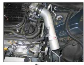
21. Install the K&N<sup>®</sup> intake tube into the silicone hose at the throttle while also installing the crankcase vent chamber into the grommet installed in the K&N<sup>®</sup> intake tube. Align the tube mounting bracket with the removed cam cover bolt location. Secure the intake tube with the cam cover bolt removed in step #12 and the hose clamp provided.
