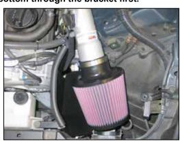
28. Install the  $K\&N^{\circledR}$  air filter onto the intake tube as shown and secure with the provided hose clamp
