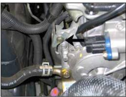
38. Remove the cam cover bolt shown. **NOTE: This bolt will not be reused.**
