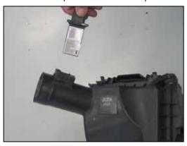
42. Remove the two screws securing the mass air sensor to the airbox assembly and then remove the mass air sensor as shown.
