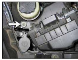
34. Remove the passenger side airbox mounting bolt shown.
