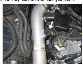
46. Reconnect the mass air sensor electrical connection.
