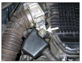
30. Remove the crankcase vent chamber mounting bolt shown.
