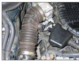
31. Loosen the spring clamp which secures the crankcase vent chamber to the passenger side intake tube and then unhook the crankcase vent chamber from the intake tube as shown.
