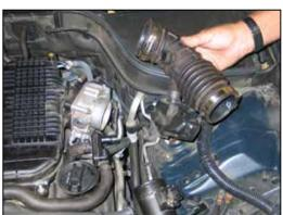
6. Release the spring clamp which secures the crankcase vent hose to the intake tube and then remove the intake tube from the vehicle.
