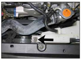
37. Remove the coolant reservoir mounting bolt shown.
