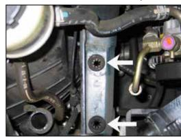
36. Remove the two passenger side airbox mounting grommets shown from the frame rail.
