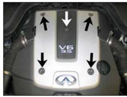
2. Remove the three bolts and two nuts that secure engine cover to the engine.
