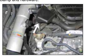
45. Connect the crankcase vent hose to the K&N<sup>®</sup> intake tube and secure with the provided hose clamp. Secure the crankcase vent chamber with the factory bolt removed during step #30.
