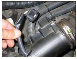
29. Disconnect the passenger side mass air sensor electrical connection and then unhook the wiring harness from the airbox.
