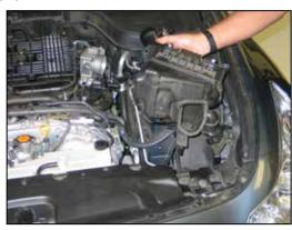
9. Remove the driver's side airbox assembly from the vehicle.
