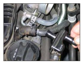
7. Disconnect the driver's side crankcase vent hose from the vent chamber as shown and then remove the crankcase vent hose from the valve cover.
