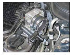
16. Install the silicone hose (08440) onto the throttle body and secure with the provided hose clamp as shown.
