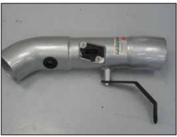
20. Install the mass air sensor into the K&N<sup>®</sup> intake tube and secure with the provided hardware.
