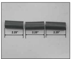
13. Cut the supplied crankcase vent hose into three 2-1/4" long sections.
