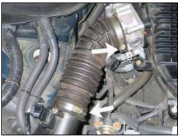
32. Loosen the two hose clamps which secure the stock intake tube.
