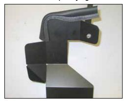
49. Install the edge trim onto the heat shield as shown.
