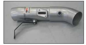
40. Attach the provided tube mounting bracket (07171) onto the  $K\&N^{\circledR}$  intake tube (27411) using the provided hardware.
