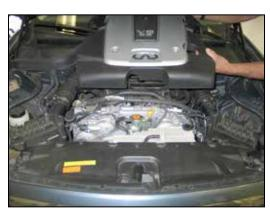
3. Lift off the engine cover as shown.
