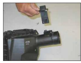
19. Remove the two screws which secure the mass air sensor into the stock airbox and then remove the mass air sensor assembly.
