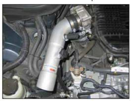
44. Install the K&N<sup>®</sup> intake tube into the silicone hose at the throttle body and align the mounting bracket with the removed bolt location from step #38. Secure the intake tube with the provided hose clamp and hardware.
