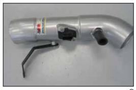
43. Install the mass air sensor into the K&N<sup>®</sup> intake tube and secure with the provided hardware.
