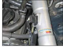
22. Reconnect the mass air sensor electrical connection.
