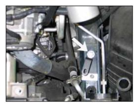
24. Insert the well nut into the airbox mounting grommet hole in the frame rail. Tighten the mounting bolt to secure the mounting bracket and well nut.
