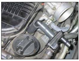
15. Install the 90° crankcase vent assembly onto the valve cover and then attach the crankcase vent chamber as shown.
