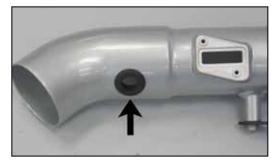
18. Install the provided grommet into the intake tube as shown.
