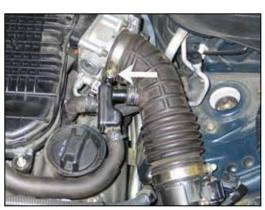
5. Loosen the two hose clamps shown that secure the driver's side intake tube.
