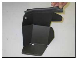
26. Install the provided edge trim onto the heat shield as shown.
