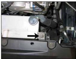
11. Remove the coolant reservoir mounting bolt shown.
