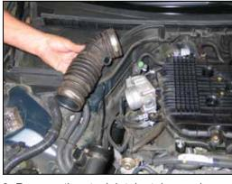
33. Remove the stock intake tube as shown.
