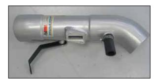
41. Install the remaining 2-1/4"long crankcase breather hose onto the  $K\&N^{\textcircled{R}}$  intake tube and secure with the provided hose clamp.
