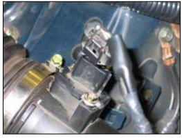
4. Disconnect the driver's side airbox mass air sensor electrical connection and unclip the wiring harness from the airbox.
