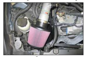
51. Install the  $K\&N^{\textcircled{R}}$  air filter and secure with the provided hose clamp.
