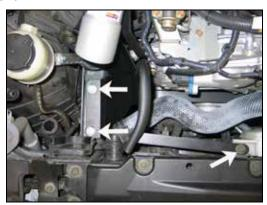
50. Set the heat shield assembly into the engine bay as shown. Secure the heat shield mounting bracket to the coolant reservoir with bolt removed in step #37. Tighten the well nut mounting bolts.
