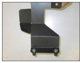
48. Install the two well nuts onto the heat shield and secure with the provided hardware.
