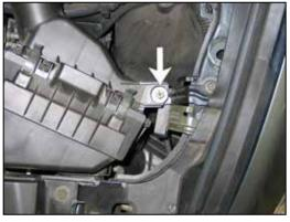
8. Remove the driver's side airbox mounting bolt shown.
