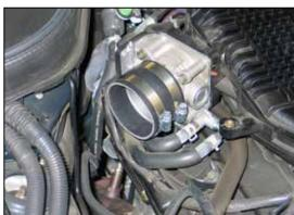
39. Install the supplied silicone hose (08440) onto the throttle body and secure with the provided hose clamp.
