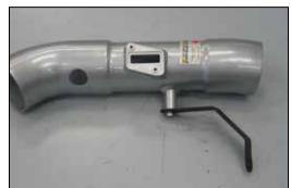
17. Attach the tube mounting bracket (07171) onto the driver's side intake tube (27412) using the supplied hardware.
