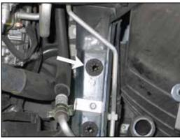
10. Remove the driver's side airbox mounting grommet shown from the frame rail.
