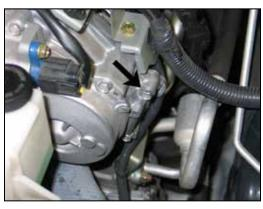
12. Remove the cam cover bolt shown. **NOTE: This bolt will be reused in a later step.**
