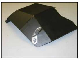
25. Attach the heat shield mounting bracket (06717) to the driver's side heat shield (07682) using the provided hardware.
