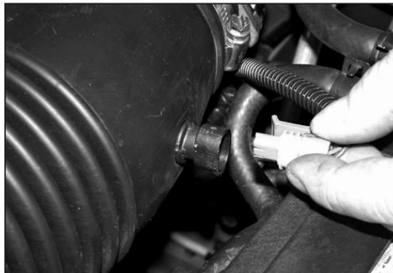
4. Release the air temp. electrical connection clip, then disconnect the electrical connection.
