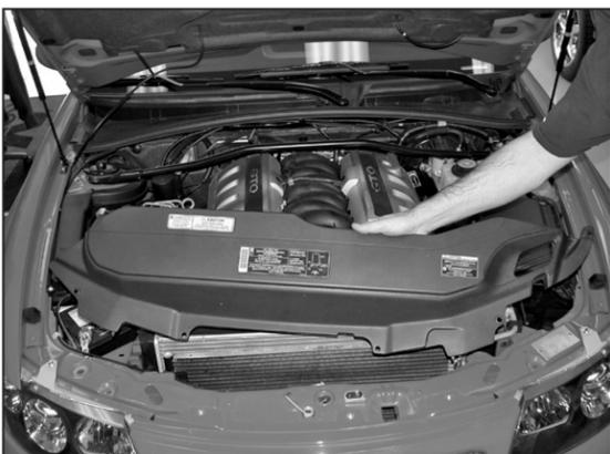
3. Lift up on the radiator cover and pull back to release from the retaining hook, then remove the cover from the vehicle.
