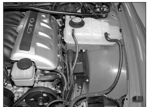
9. Reinstall the coolant reservoir onto the mounting studs as shown.
