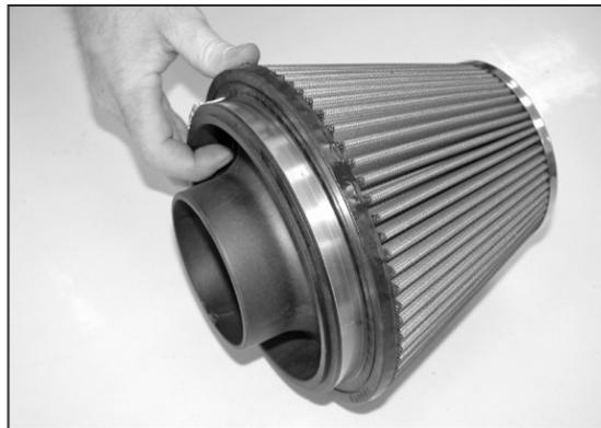
19. Install the filter adapter into the K&N® filter as shown. Secure with the provided hose clamp.
