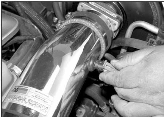
31. Reconnect the temperature sensor electrical connection.
