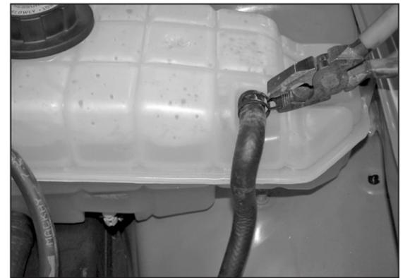
21. Make sure pressure is released from radiator cap before loosening spring clamp. Re-install the coolant reservoir back onto the two retaining studs, then, using a pair of pliers, loosen the spring clamp on the coolant reservoir hose. Rotate the coolant hose 90 degrees down as shown. Then resecure with the stock clamp.
