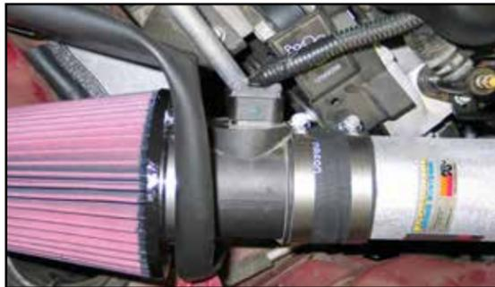
28. Re-connect the mass air sensor as shown.
