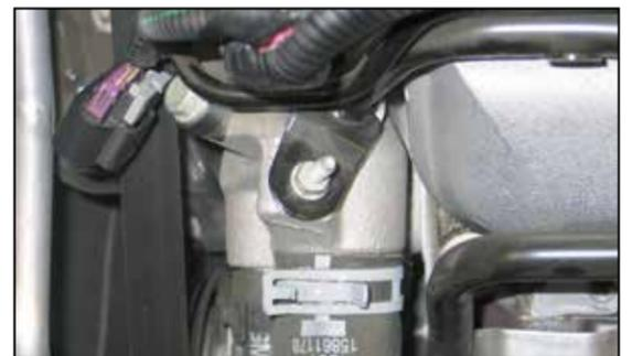
20a. On vehicles equipped with the above style heater hose tube, remove the mounting bolt shown.
