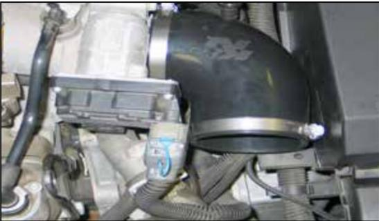
14. Install the provided silicone hose (08629) onto the throttle body with the provided hose clamp.
