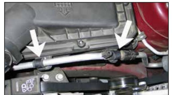
8. Remove the two clamps securing the A/C line to the stock air box.
