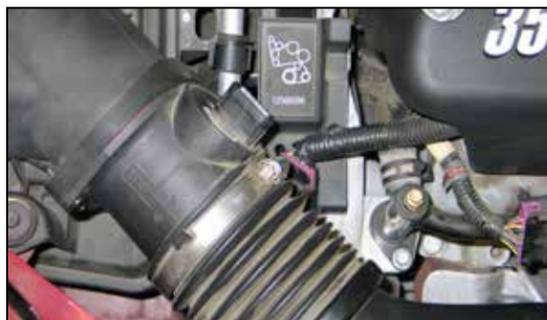
5. Loosen the hose clamp that secures the stock intake to the mass air sensor.
