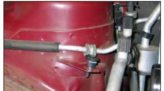
23. With the bolt removed in step #9 and spacer (#07849) secure the A/C line to the inner fender as shown.
