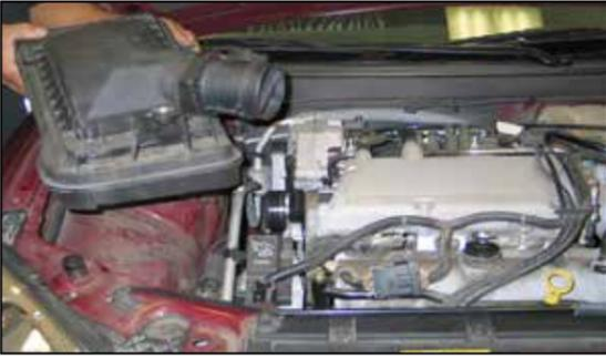
10. Remove the stock air box from the vehicle.
