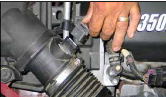
2. Depress the locking tab and disconnect the mass air sensor electrical connection.
