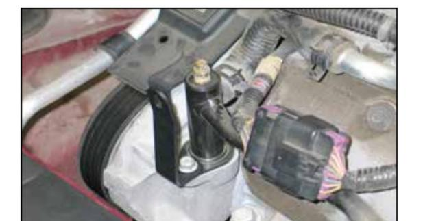
21. Install the correct tube mounting bracket (06496 or 070049) to match the style heater hose tube as shown in the above photos and secure with the factory bolt removed in step #20a.
