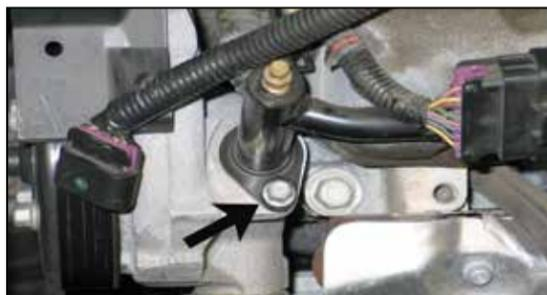
20. On vehicles equipped with the above style heater hose tube, remove the mounting bolt shown.
