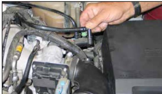
4. Remove the crank case vent tube from the stock intake tube.
