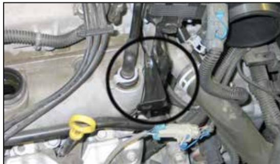
19. Install "L" bracket (#070742) to the 1/4" id hole in the engine lifting bracket using the provided hardware as shown.
