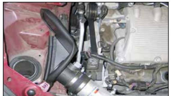
24. Install the mass air sensor and heat shield assembly. Secure with the provided hose clamp as shown.
