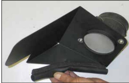
16. Install the provided edge trim (short) onto the heat shield as shown.
