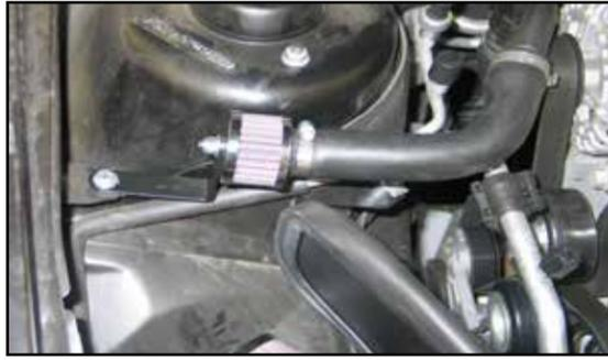
26b. Secure the air injection filter assembly to the air box mount with the provided hardware and then attach the air injection hose to the filter and secure with the provided hose clamp as shown.
