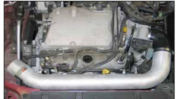
22. Install the K&N® Intake Tube into the silicone hose at the throttle body and align the intake tube with the mounting brackets installed in the previous step. Secure the intake tube with the provided hardware and hose clamp.
