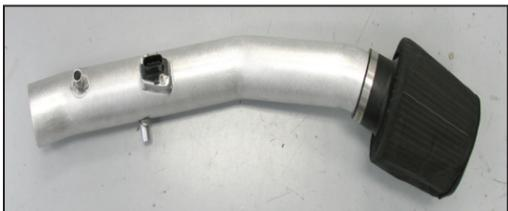
15. Install the K&N® filter assembly onto the K&N® intake tube and secure with the provided hose clamp.
