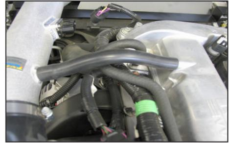
21. Install the supplied crankcase vent hose onto the valve cover and onto the intake tube as shown. **NOTE: Some trimming of the hose may be necessary.**
