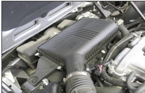
6. Release the six upper airbox mounting clips.
