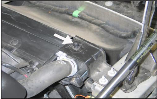
10. Remove the right lower airbox mounting studs shown from the bracket.
