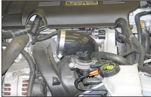
16. Install the provided silicone elbow hose onto the throttle body and secure with provided hose clamp.
