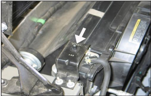
11. Remove the left lower airbox mounting studs shown from the bracket.
