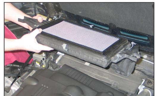
9. Pull up firmly to release the lower airbox housing from the mounting grommets and then remove the lower airbox from the vehicle.
