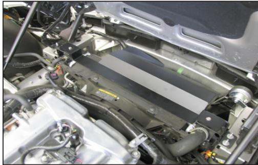
17. Install the heat shield assembly and secure to the airbox mounting points, then secure with the provided hardware.
