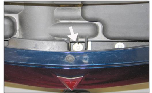
8. Remove the front lower airbox mounting bolt shown.
