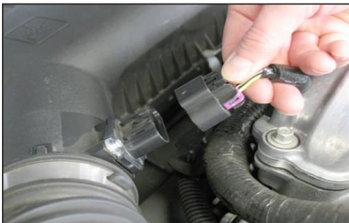
3. Depress the locking tab and then disconnect the mass air sensor electrical connection.
