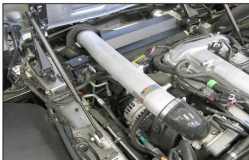
20. Install the K&N® intake tube assembly into the silicone hose at the throttle body and align with the mounting bracket installed in the previous step. Secure the tube with the hose clamp and hardware provided.
