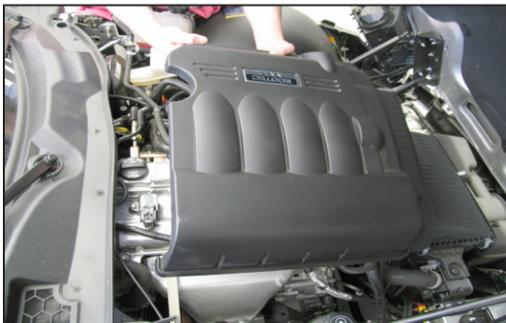
2. Lift firmly on the engine cover to dislodge it from the mounting grommets and then remove the engine cover assembly.
