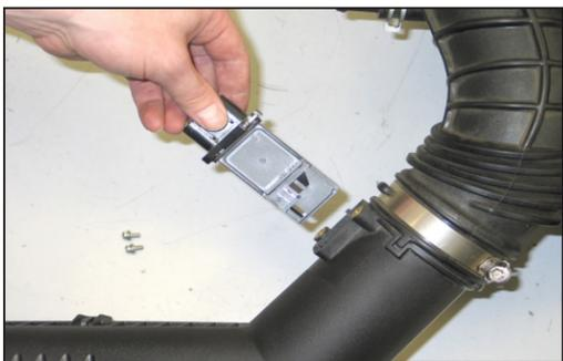
12. Remove the two screws securing the mass air sensor to the stock intake tube and then remove the mass air sensor as shown.
