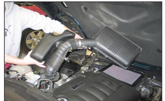
7. Firmly lift up the intake tube and upper airbox to release it from the mounting grommets and then remove the assembly from the vehicle.
