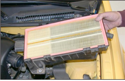
10. Remove the lower air cleaner assembly as shown.
