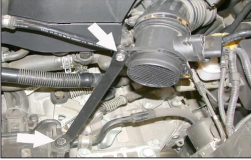
29. Secure the provided bracket to the mass air sensor using the provided hardware, then secure the other end to the battery tray using the stock air cleaner bolt as shown.
