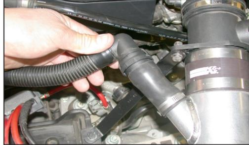
35. Reconnect the hard line to the plastic fitting as shown.
