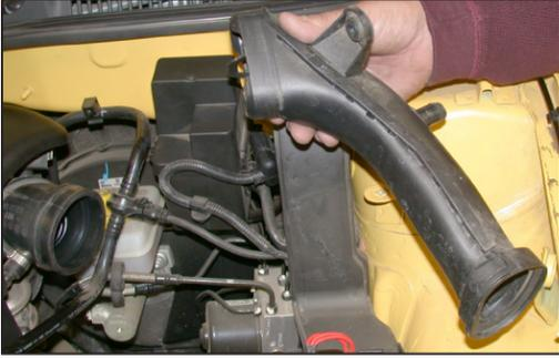
11. Remove the nut that secures the air inlet duct, then remove the air inlet duct as shown.
