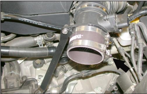
30. Install the silicone hose and hose clamps onto the mass air sensor but do not tighten at this time.
