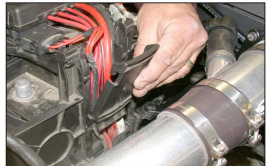
44. Slide the rear battery harness cover back onto the battery cover as shown.
