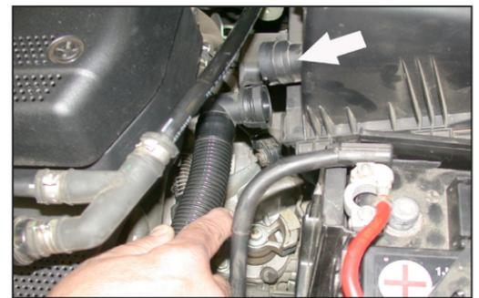
7. Disconnect the air pump vent hose as shown.
