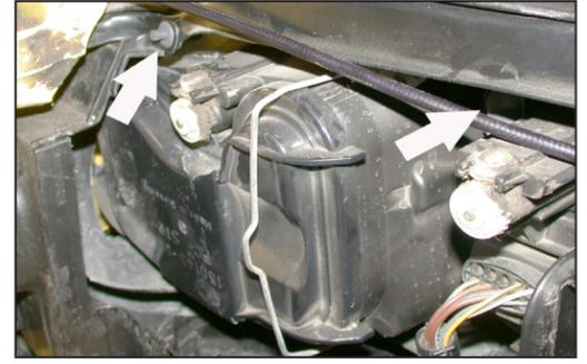
22. Remove the two upper plastic rivets from the inner plastic headlight cover as shown.
