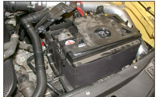
42. Reinstall the secondary battery cover as shown.
