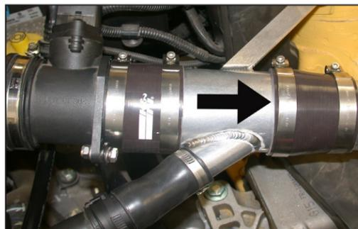
38. Slide the hose over the short ram tube, adjust for best fit and clearance and tighten all hose clamps and hardware as shown.
