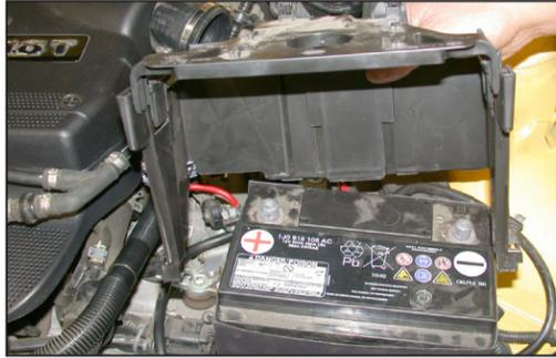
18. Remove the battery cover as shown.
