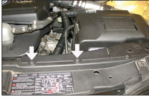
49. Reinstall the inner core support cover as shown.
