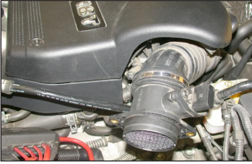
28. Reinstall the mass air sensor into the stock rubber intake hose as shown, but do not tighten at this time.
