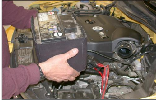
19. Remove the battery as shown.
