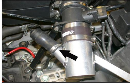
34. Slide the silicone hose onto the vent of the K&N® intake tube and secure with the provided hose clamp as shown.
