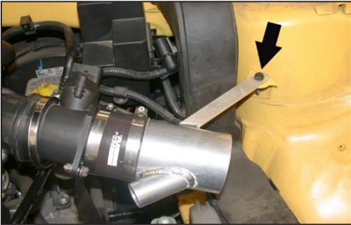
31. Slide the short K&N® intake tube into the silicone hose and secure the tube bracket to the original air cleaner mounting hole using one of the air cleaner bolts removed earlier.
