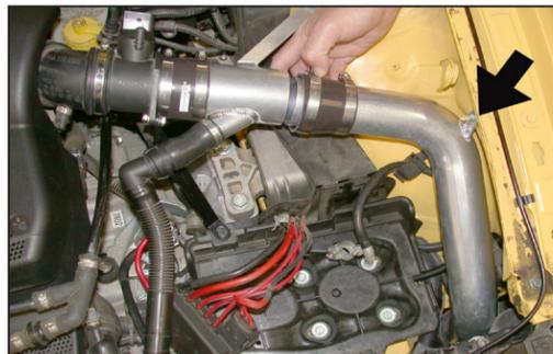
37. Slide the cold air tube into the hole in the inner fender, then, line up the bracket with the stud on the inner fender and secure with the provided hardware as shown.
