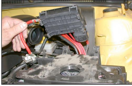
16. Slide the battery fuse/harness assembly backwards, then upwards as shown, and pull the battery fuse/harness assembly out of the way.
