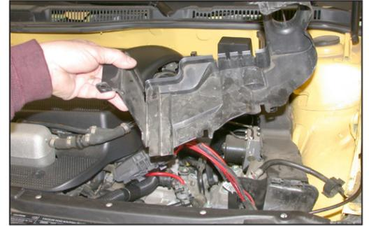
24. Remove the inner plastic headlight cover as shown.
