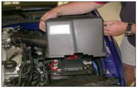
3. Unclip the battery cover and remove as shown.
