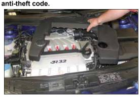
2. Pull firmly upwards to remove the engine cover
