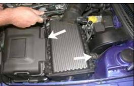
5. Remove the two air cleaner bolts as shown.
