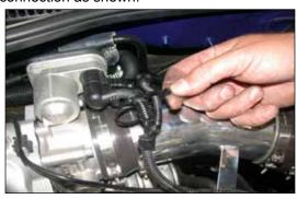
23. Zip-tie the crank case vent switch to the throttle control connection as shown.
