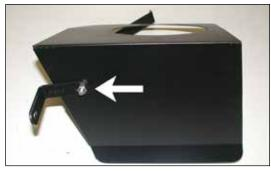
17. Install the "L" bracket onto the heat shield using the provided hardware as show, but do not tighten completely at this time.
