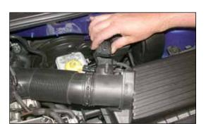
4. Disconnect the mass air sensor electrical connection as shown.
