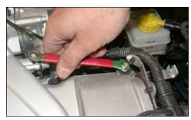
11. Loosen the nut on the cam cover but do not remove as shown.
