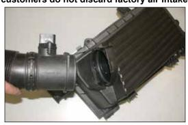
9. Remove the mass air sensor from the air cleaner assembly as shown.
