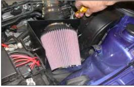
20. Install the air filter and secure with the provided hose clamp.
