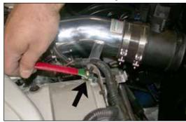
19. Adjust the tube for best fit and clearance and tighten the nut on the cam cover as well as the hose clamps on the intake tube as shown.
