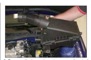
8. Depress the hose clamp to remove the stock intake tube from the throttle body, then, remove the complete air cleaner assembly as shown. NOTE: K&N Engineering, Inc., recommends that customers do not discard factory air intake.
