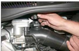
7. Remove the crank case vent hose from the intake tube as shown.
