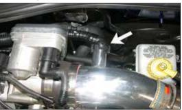
21. Reconnect the crank case vent hose to the vent on the K&N® intake tube.
