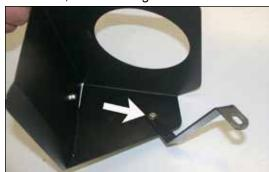
16. Install the "Z" bracket onto the heat shield using the provided hardware as show, but do not tighten completely at this time.
