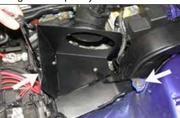
18. Install the heat shield into the vehicle and secure it using the stock air cleaner bolts, adjust for best fit and clearance and tighten all hardware.
