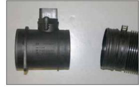
10. Remove the intake tube from the mass air sensor as shown.
