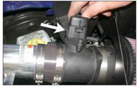
22. Reconnect the mass air sensor electrical connection as shown.
