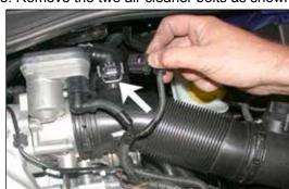
6. Disconnect the crank case vent switch as shown.
