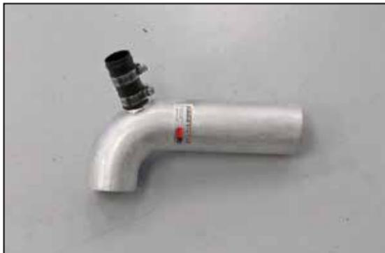
15. Install the secondary air fitting onto the K&N® intake tube as shown.
