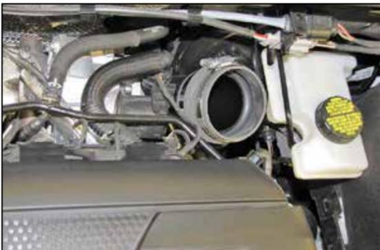
12. Install one of the provided coupling hoses (08185) onto the turbo inlet and secure with the provided hose clamp.
