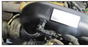
22. Reconnect the inlet air temperature sensor electrical connection.
