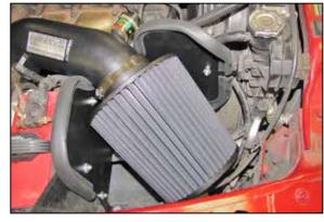
21. Install the K&N® air filter onto the K&N® intake
