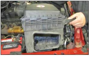
6. Lift up the air box to dislodge it from the mounting grommets and then remove the air box from the vehicle.
