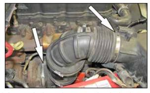
3. Loosen the hose clamps securing the intake hose to the turbo inlet and to the factory air box.
