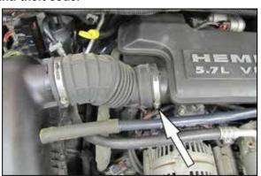
2. Loosen the hose clamp securing the factory intake tube to the intake plenum.
