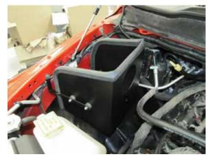
19. Install the heat shield assembly into the vehicle and secure to the bracket previously installed, to the inner fender and rubber mounted stud.
