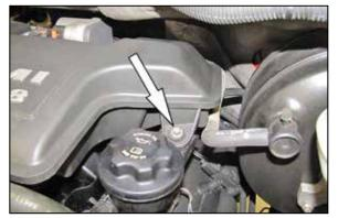
6. Loosen the remaining bolt securing the intake plenum.
