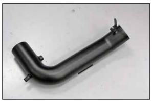
21. Install the tube mounting bracket (070049) onto the rubber mounted stud as shown.
