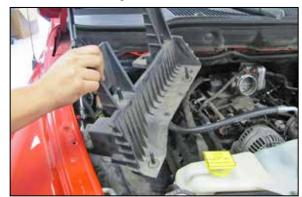
10. Remove the four bolts that secure the air filter mounting bracket and then remove the bracket from the vehicle.
