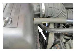
3. Disconnect the crank case vent hose from the air
