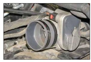
25. Install the provided coupling hose (08698) onto the throttle body and secure with the provided hose
