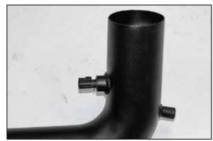
24. Install the inlet air temperature sensor into the silicone hose installed in step #21.
