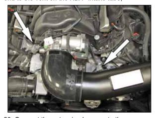
20. Connect the extension harness to the factory engine harness and then into the inlet air temperature.
