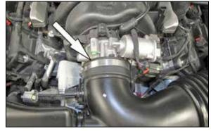
4. Loosen the hose clamp that secures the intake hose to the throttle body and then pull the intake tube from the throttle body.
