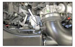
3. Release the locking tap and then disconnect the inlet air temperature sensor electrical connection.
