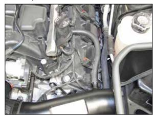
19. Install the provided crank case vent hose onto the fitting on the engine and then connect the open end to the vent on the K&N<sup>®</sup> intake tube,
