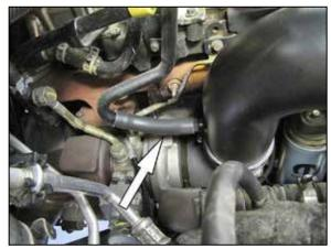
25. Install the provided crank case vent hose onto the fitting installed into the K&N® intake tube and then attach the open end to the factory vent pipe. NOTE: Some trimming of the hose may be necessary.
