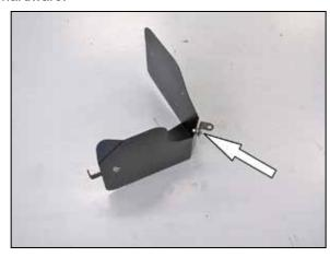
11. Install the tube mounting bracket (070712) onto the heat shield as shown using the provided hardware and spacer.
