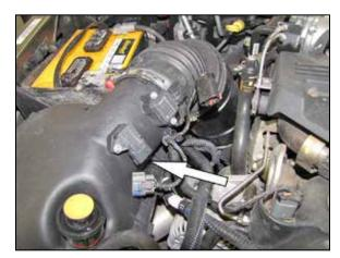
3. Disconnect the inlet air temperature sensor electrical connection and then unhook the wiring harness from the air box.
