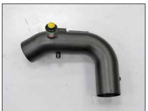
21. On vehicles equipped with a filter minder, install the factory grommet and filter minder into the K&N® intake tube as shown.
