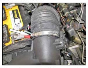
4. Loosen the hose clamp which secures the intake hose to the upper air box housing.
