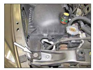
5. Loosen and remove the nut which secures the air box to the core support.
