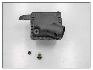
19. On vehicles equipped with a filter minder, remove the filter minder and factory grommet from the air box as shown.
