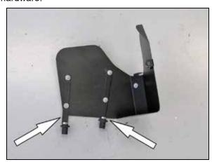
13. Install the heat shield mounting bracket assemblies (07159) onto the heat shield as shown using the provided hardware.
