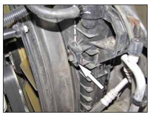
16. Remove the fan shroud bolt shown.
