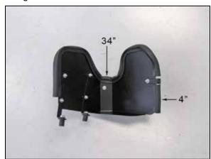
15. Install the edge trim onto the heat shield as shown.
