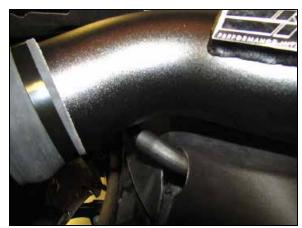
27. Connect the crank case vent hose to the fitting installed into the K&N® intake tube and secure with the provided hose clamp.
