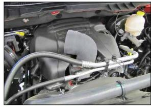
21. Install the provided silicone hose (084086-1) onto the throttle body and secure with the provided hose clamp.
