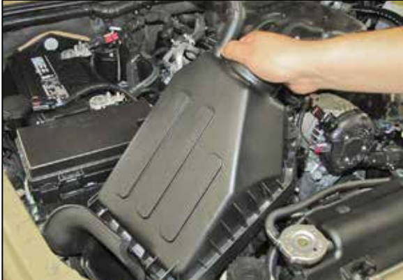
8. Lift up and remove the air filter housing from the vehicle.
