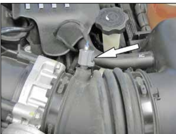
2. Disconnect the inlet air temperature air sensor electrical connection.
