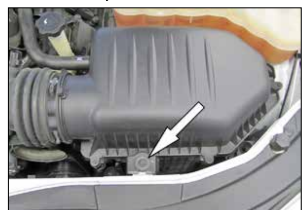
6. Remove the bolt which secures the air box to the core support.
