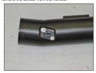
19. Install the mass air sensor into the K&N<sup>®</sup> intake tube and secure with the provided hardware.
