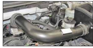
20. Install the K&N® intake tube into the 90° elbow hose and then into the hump hose, align for best fit and then secure with the provided hose clamp.
