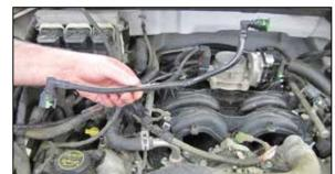
9. Release the crank case vent hose from the valve cover port and then remove the crank case hose from the vehicle.
