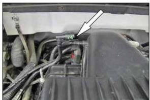
3. Disconnect the crank case vent line as shown.
