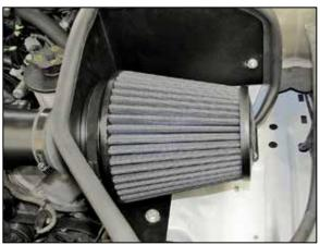
23. Install the  $K\&N^{\otimes}$  air filter onto the filter adapter and secure with the provided hose clamp.
