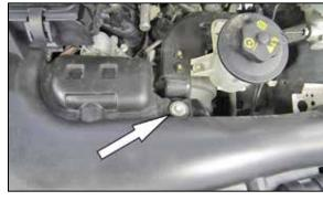
5. Remove the bolt shown securing the intake snorkel to the bracket.
