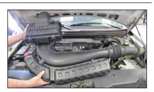
7. Remove the complete air box and intake snorkel assembly as shown.
