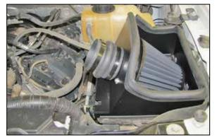
15. Install the provided hump coupling hose (5-580) onto the filter adapter and secure with the provided hose clamp.
