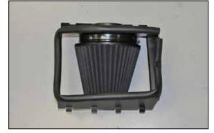
11. Install the air filter onto the filter adapter and secure with the provided hose clamp.
