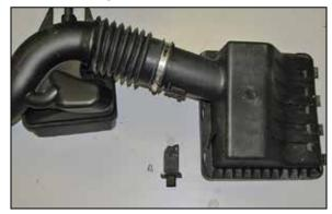
17. Remove the two screws securing the mass air sensor and then remove the mass air sensor from the stock intake tube as shown.
