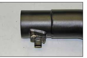
18. Install the mass air sensor into the K&N $^{\otimes}$  intake tube and secure with the provided hardware.
