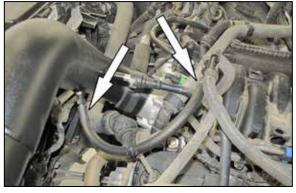
21. Install the provided EVAP vent hose onto the 3/8" fitting installed in the intake tube and then attach the open end to the EVAP check valve.
