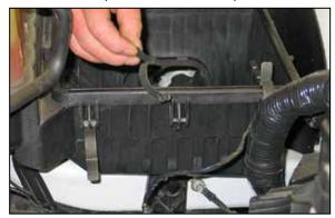
12. Remove the center air box retaining clip.
