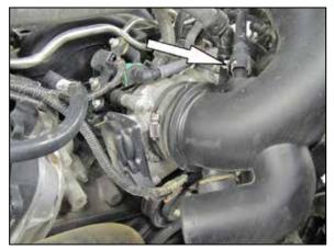
3. Rotate the locking tab and then unhook the crank case vent hose from the factory intake tube.
