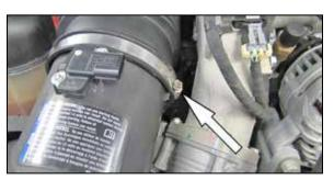
3. Loosen the hose clamp securing the factory intake tube to the air box.
