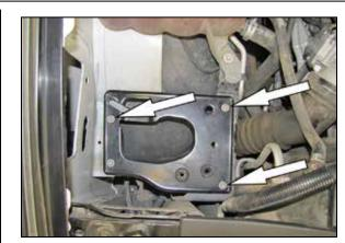
6. Remove the three bolts shown securing the air filter mounting plate.
