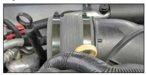
15. Install the provided hump hose (08633) onto the turbo inlet and secure with the provided hose clamp.
