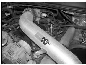
20. Slide the K&N® intake tube into the silicone hose on the throttle body and secure the bracket to the alternator using the stock bolt removed in step
