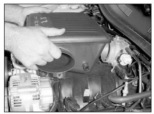
8. Pull firmly upward and remove the intake tube assembly.
