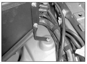
16. Attach the "L" twist bracket to the existing airbox mounting point on the inner fender apron using the hardware provided.
