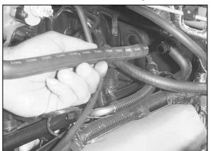
9. Detach the OE crankcase vent hose from the "T" fitting.
