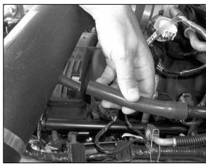
25. On 2003 models slide the silicone hose from step 24 onto the crank case vent hard line as shown.
