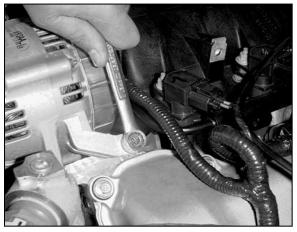
18. Loosen and remove the alternator retaining bolt.
