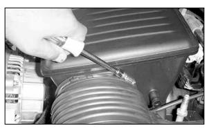
3. Loosen the hose clamp on the intake hose at the intake tube.
