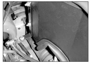
17. Attach the "L" bracket to the radiator mounting bracket using the hardware provided.
