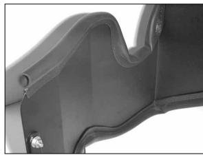
14. Install the trim seal onto the heat shield as
