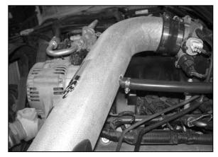
26. On 2003 models connect the crank case vent hose to the K&N<sup>®</sup> intake as shown.
