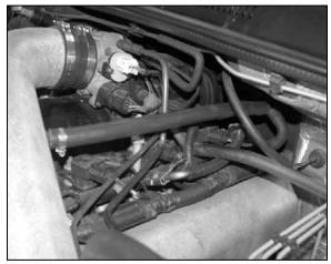
23. Connect the other end of the silicone hose to the vent on the K&N<sup>®</sup> intake tube as shown.
