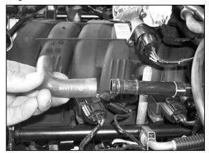
9a. On 2003 models, detach the 90 degree hose from crankcase vent as shown.
