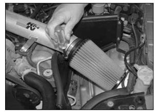
27. Install the K&N<sup>®</sup> air filter on the K&N<sup>®</sup> intake tube and secure with the provided hose clamp as
