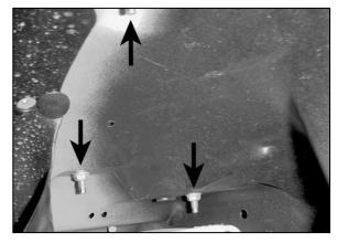
10. Loosen and remove the 3 nuts that retain the airbox base to the inner fender apron.
