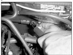
22. Attach the vent hose provided to the "T" fitting.
