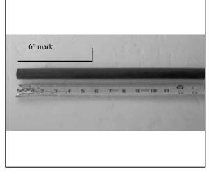
24. On 2003 models, cut 6 inches of the provided silicone hose as shown.
