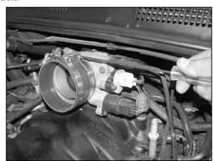
19. Install the provided silicone step hose and hose clamps onto the throttle body as shown.
