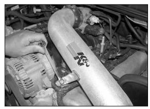
21. Adjust everything for best fit and clearance then tighten the alternator bolt as shown.
