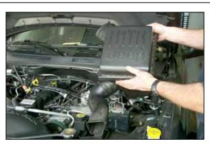
cleaner assembly from underneath the vehicle, then, remove the air cleaner assembly as shown.
