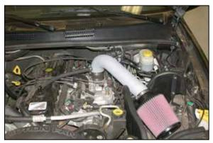
13. Reconnect the vehicle's negative battery cable. Double check to make sure everything is tight and properly positioned before starting the vehicle. NOTE: Drycharger® air filter wrap; part # RX-4730DK is available to purchase separately. To learn more about Drycharger® filter wraps or look up color availability please visit http://www.knfilters.com.
