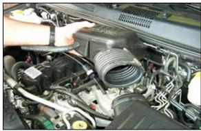
4. Loosen the hose clamp at the air cleaner lid and at the throttle body, then, remove the resonator and bellows assembly as shown.
