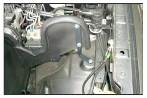
8. Install the heat shield into the vehicle and secure the twist bracket to the original air cleaner mounting hole using the provided hardware.
