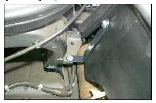
9. Secure the "L" bracket to the hole on the flange/ tab on the radiator core support using the provided hardware.
