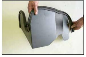
6. Install the provided trim seal onto the heat shield as shown.
