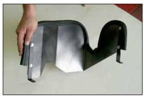
7. Using the provided hardware install the two brackets onto the heat shield as shown.
