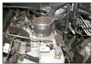
10. Install the provided silicone hose and hose clamps onto the throttle body as shown.
