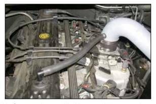
12. Connect the provided hose to the vent on the valve cover, then, connect the other end to the vent on the K&N<sup>®</sup> intake tube as shown.
