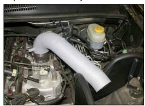
11. Install the K&N<sup>®</sup> intake tube into the silicone hose as shown, but do not tighten completely as some adjustment may be necessary.
