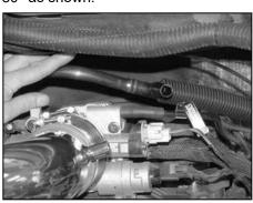
37. Reinstall the vent tube assembly into the rubber fittings in each valve cover so that the "T" fitting is now on the drivers side of the engine facing forward.
