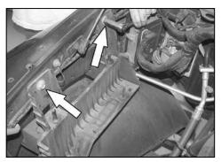
10. Remove the air cleaner support bracket, that is secured by the two bolts on the upper fender and two bolts on the lower fender.
