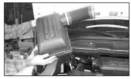
3. Lift up firmly to release the air box from mounting studs, then remove completely.
