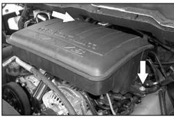
5. Remove the two 10mm bolts that retain the resonator box onto the engine.
