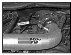
33b. Connect the open end of the inlet air temperature sensor extension harness into the inlet air temperature sensor as shown.
