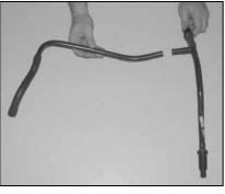
35. Cut the crank case vent tube 1" from the "T" fitting as shown.
