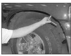
11. Reinstall the inner fender removed in step #9. **NOTE: Two of the retaining bolts will not be used.**
