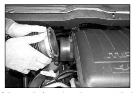
2. Loosen the hose clamp that connects the intake tube to the resonator box then remove the intake tube.
