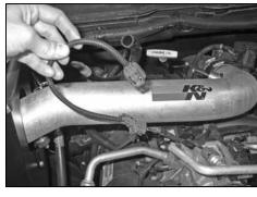
33a. On 2008 and later model year vehicles, connect the provided inlet air temperature sensor extension harness into the factory connection as shown.
