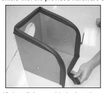
18. Install the provided edge trim onto the heat shield and trim to fit.
