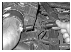
31. On vehicles with the crank case vent hose connected to the "T" on the drivers side of the engine, install the 90° vent fitting into the stock crank case hose as shown.
