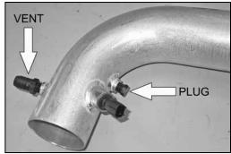
25a. On 2002-2007 model year vehicles, install the 1/4"npt vent fitting and plug as shown.
