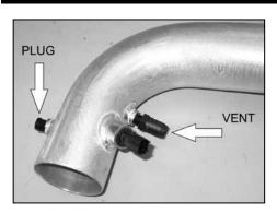
25b. On 2008 and later model year vehicles, install the 1/4"npt vent fitting and plug as shown.
