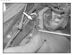
12. Remove the bolt that secures the computer to the inner fender as shown.
