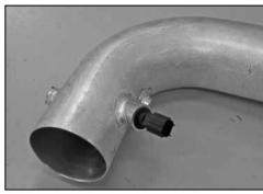
25. On vehicles equipped with an air temperature sensor, install the air temperature sensor into the silicone hose as shown.
