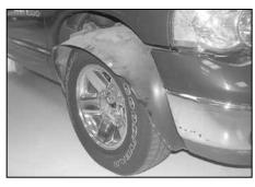
9. Loosen and remove the eight bolts that secure the inner fender valance; lower the valance down as shown.
