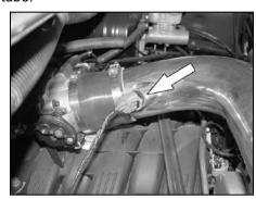
33. On 2002-2007 model year vehicles, reconnect the inlet air temperature sensor electrical connection as shown.
