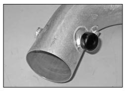
21. On vehicles not equipped with an air temperature sensor, install the provided cap plug and secure with the provided hose clamp.
