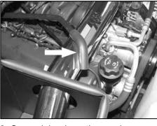
39. On models where the crank case vent hose is connected to the passenger side valve cover, remove the factory 90° coupling hose from the plastic vent tube.
