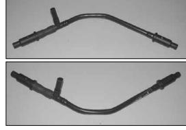
36. Rotate the long side of the vent tube assembly 180° as shown.
