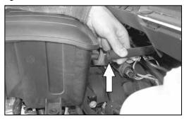
7. On 2002-2007 model year vehicles, disconnect the crank case vent hose from resonator as shown, then remove resonator from vehicle.
