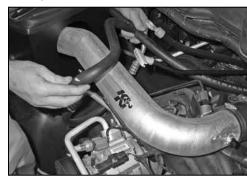
34. On models where the crank case vent hose is connected to the "T" on the passengers side of the engine, remove the complete vent tube assembly from the rubber fittings in each valve cover as shown.
