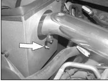
29. Line up the angle bracket with the heat shield and secure with the provided hardware as shown.
