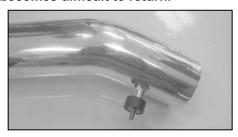
26. Install the rubber mounted stud into the threaded boss on the K&N® intake tube as shown.
