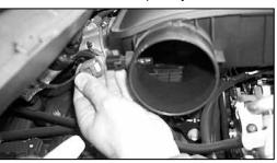
4. On models that come equipped with air temp sensors, unplug the air temp. sensor electrical connection as shown.
