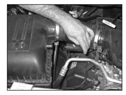
2a. On 2008 and later model year vehicles, disconnect the crank case vent hose from the air box as shown.
