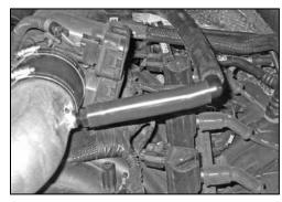
32. Install the provided silicone hose onto the 90° vent, then connect the other end of the silicone hose onto the vent attached to the K&N® intake tube.
