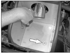
30. Install the remaining hardware, adjust the heat shield for best fit and clearance; tighten all hardware as shown.
