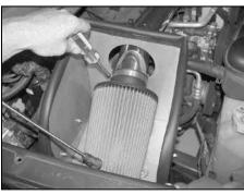
42. Install the air filter and secure with the provided hose clamp as shown.
