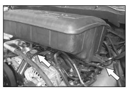
6. Pull up firmly to release the resonator from the engine.
