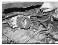
20. Install the silicone hose and hose clamps onto the throttle body and tighten as shown.
