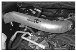
28. Install the K&N® intake tube into the silicone hose at the throttle body and align the mounting bracket with the heat shield. Secure the intake tube with the hose clamp and hardware provided.
