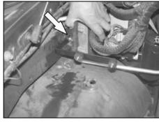
14. Secure the angle bracket assembly to the threaded hole from step 12 and secure with the stock bolt.
