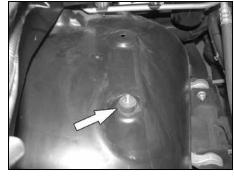
15. Install the provided rubber mounted stud into the existing hole on the inner fender and secure from underneath the inner fender with the provided rubber washer, fender washer and nylock nut as shown.
