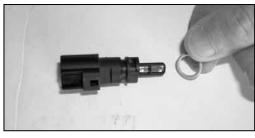
24. Remove the O-ring from the air temp. sensor as shown.
