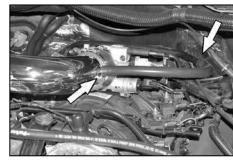
40. On models with the crank case vent tube connected to the passenger side valve cover, connect the provided silicone hose to the factory vent tube. Then, route the crank case vent tube assembly behind the throttle body as shown. Connect the open end onto the K&N® intake tube.
