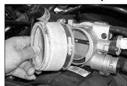
8. On 2002-2007 model year vehicles, loosen the hose clamp that retains the rubber hose to the throttle body and remove as shown.
