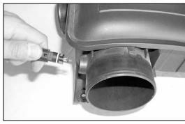
23. On models that come equipped with temp sensors, remove the air temp sensor from the resonator as shown.
