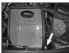
19. Install the heat shield assembly onto the rubber mounted studs and line up the "L" bracket with the threaded hole from step 12 and secure with the stock bolt as shown.
