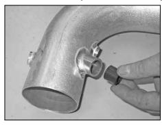
22. On vehicles equipped with an air temperature sensor, install the provided silicone hose into the vent on the K&N® intake tube as shown.
