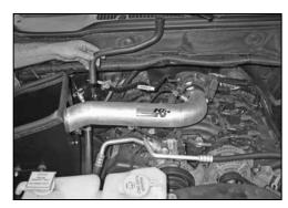
41a. On 2008 and later model year vehicles, remove the crank case vent hose from the passenger side valve cover as shown.
