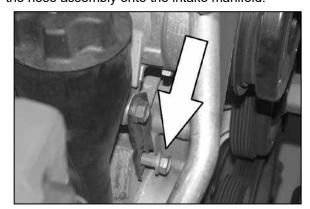
8. Remove the lower A/C bracket bolt shown with a 15mm socket.
