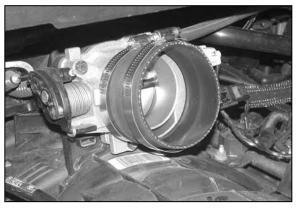
14. Install the silicone hose (084091) onto the throttle body and secure with the provided hose clamps.
