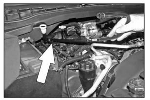
7a. On 2006 and later vehicles, disconnect the crankcase vent tube from the rear of the intake manifold.
