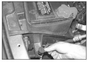
12. Install the 3/8" threaded insert provided into the airbox mounting grommet hole vacated in step #11.
