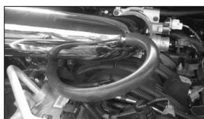
22a. On 2006 and later vehicles connect the crankcase vent hose installed in step #7c to the K&N® intake tube as shown.
