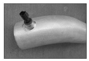
18. Install the air temperature sensor into the vent on the K&N® intake tube as shown.
