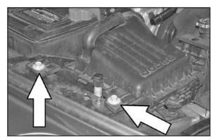
4. Remove the two airbox retaining bolts.
