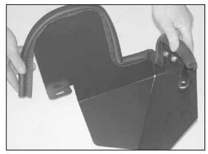
10. Install the provided edge trim onto the heat shield.
