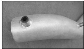
17. Install silicone hose into fitting on the  $K\&N^{\otimes}$  intake tube as shown.
