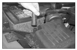
2a. On 2006 and later vehicles, disconnect the crankcase vent tube from the airbox lid as shown.
