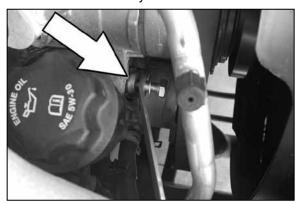
20. Line up the bracket with upper alternator mount and install the provided spacer, washer and hex
