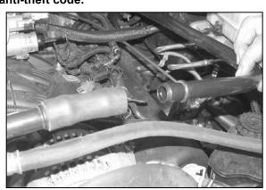
2. On 2005 and earlier vehicles, disconnect the crankcase vent tube from the vent hose junction above the alternator.
