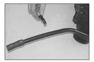
23. On 2005 and earlier vehicles remove the crankcase vent tube mounting clip from the crankcase vent tube on the airbox as shown.
