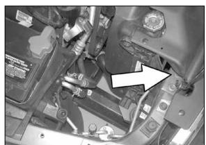
11a. On 2009 and later vehicles, the mounting bolt used has been eliminated. The heat shield bracket will need to move to the left mounting bolt which is under the radiator cover. It may be necessary to loosen the radiator cover.
