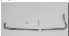
7b. On 2006 and later vehicles, measure 12" from the crankcase check valve and cut the crankcase vent tube as shown.
