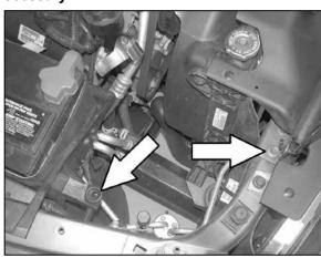
11. On 2008 and earlier models, remove the core support mounting bolt shown with a 13mm wrench, and pull out the stock airbox mounting grommet shown.
