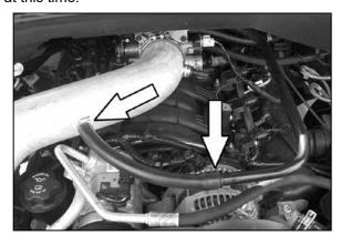
22. On 2005 and earlier vehicles connect the provided silicone hose to the crankcase vent hard line, then connect the other end to the vent on the K&N® intake tube as shown.
