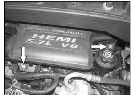
8. Remove the two 10mm resonator retaining bolts, then remove the resonator from the vehicle.
