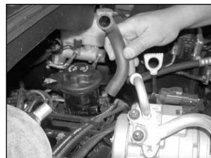
23. Remove the stock crank case vent hose as shown.
