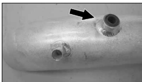
19. Install the silicone hose into the fitting on the intake tube as shown.
