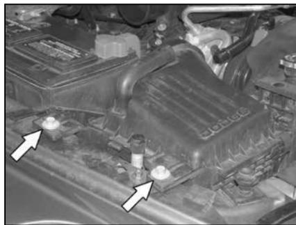
4. Remove the two air box retaining bolts.
