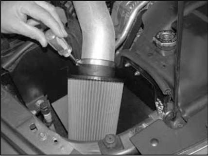
26. Install the K&N® air filter and secure with the provided hose clamp as shown.
