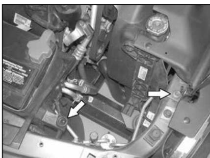
13. Remove the core support mounting bolt shown with a 13mm wrench, and pull out the stock air box mounting grommet shown.
