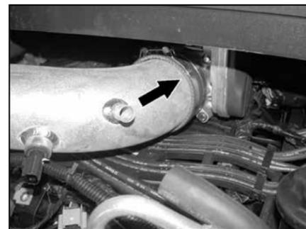
21. Slide the intake tube into the silicone hose on the throttle body as shown.
