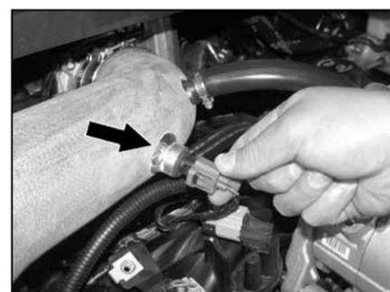
25. Reconnect the air temperature sensor electrical connection as shown.
