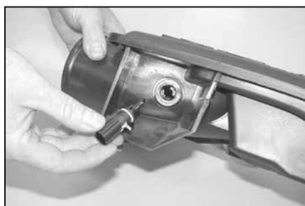
17. Twist the temp sensor counter clockwise to unlock and remove the temp sensor from the resonator.
