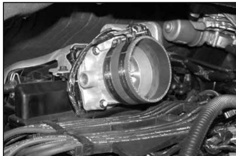
16. Install the silicone hose (08698) onto the throttle body and secure with the provided hose clamp.
