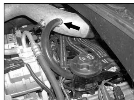
24. Connect the provided silicone hose to the crank case vent on the oil fill tube, then, connect the other end to the vent on the intake tube as shown. **NOTE: Cut 1 inch off the provided silicone hose.**
