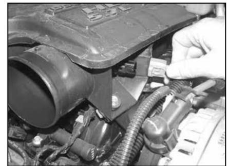
7. Depress the locking tab on the air temp sensor and disconnect its electrical connection.
