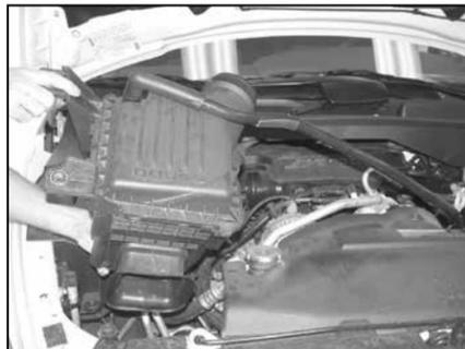
5. Pull up firmly to dislodge the air box from the mounting grommet, and remove the air box from the vehicle.
