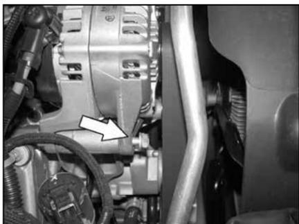
10. Loosen the bolt on the alternator but do not remove as shown.
