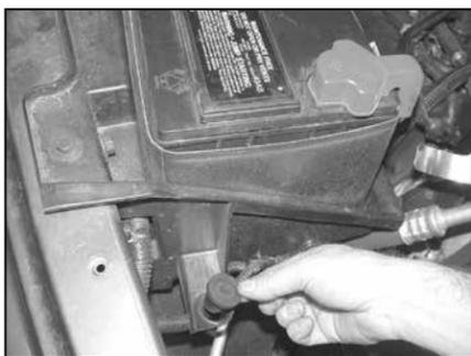
14. Install the 3/8" threaded insert provided into the air box mounting grommet hole vacated in step #14.
