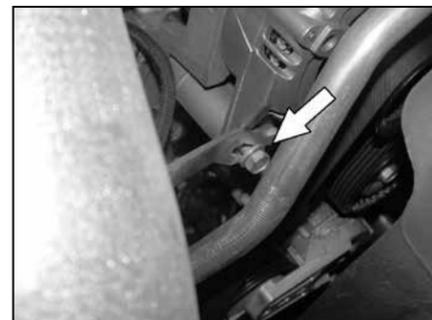
22. Rotate the bracket onto the hex bolt from step 10 and snug the bolt, but do not completely tighten at this time.
