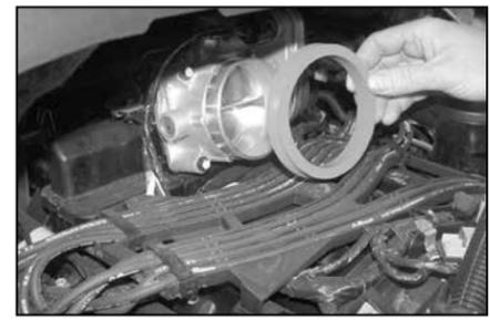
9. Remove the resonator silicone gasket from the throttle body.
