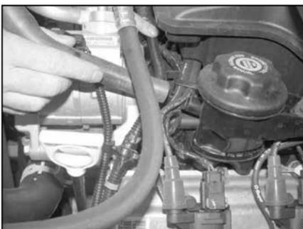
2. Disconnect the crank case vent hose at the oil filler stand off as shown.
