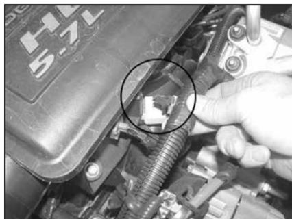
6. Unclip the engine wire harness clip from the resonator box as shown.
