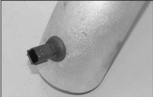
29. Install the air temperature sensor into the grommet in the K&N® intake tube as shown.
