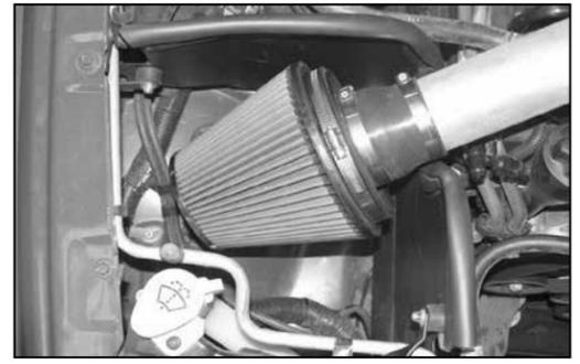
39. Install the air filter assembly onto the intake tube and secure with the provided hose clamp.
