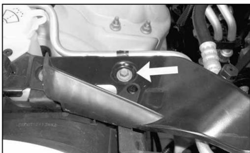
14. Remove the 6mm bolt from core support.
