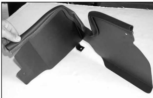
17. Install edge trim onto heat shield as shown.
