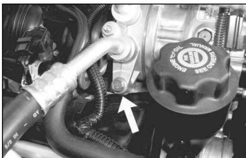
21. Remove the A/C compressor-mounting bolt.
