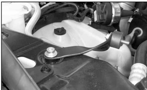
16. Install the bracket onto core support with the provided allen bolt as shown.
