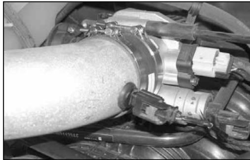
35. On vehicles equipped with the air temperature sensor, reconnect the sensor electrical connection.
