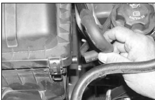
6. Disconnect the crank case vent hose from the factory air box as shown.
