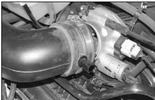
5. On vehicles not equipped with an intake resonator, loosen the hose clamp which secures the intake tube to the throttle body and then disconnect the intake tube from the throttle body as shown.
