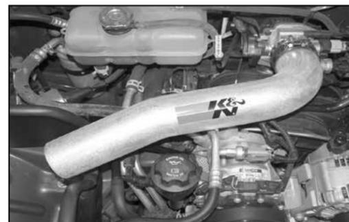
24. Install the K&N® intake tube into the silicone hose at the throttle body and align with the mounting bracket installed in step #22.
