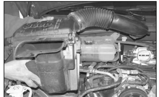
7. Firmly lift up to disengage the air box from the mounting grommets and remove the air box from the vehicle.
