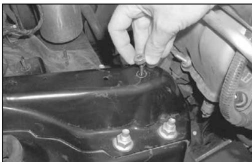
19. Vehicles that do not come equipped with cruise control, install the provided spacer and washer onto the stud as shown.
