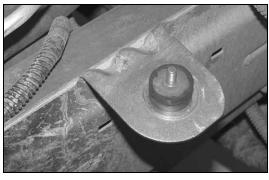
19. Using the two fender washers and one rubber washer, install the 6mm male/female rubber mounted stud onto the lower airbox mount as shown.
