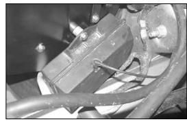
22. On vehicles equipped reconnect the vacuum reservoir vacuum line.
