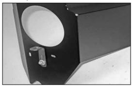
11. Install the tube mounting bracket (07131) onto the heat shield with the provided hardware as shown.
