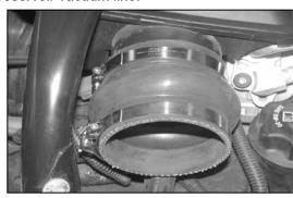
23. Install the silicone hose (084056) onto the intake plenum and secure with the provided hose clamp as shown.
