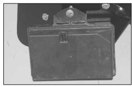
17.On vehicles equipped with vacuum reservoir, using the provided spacer, install the vacuum reservoir onto the heat shield as shown.
