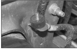
20. Install the 6mm male/male rubber mounted stud onto the upper airbox mount as shown.
