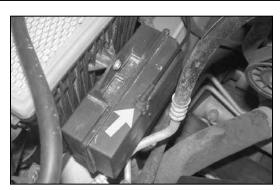
4. On vehicles equipped disconnect the vacuum canister hose shown.
