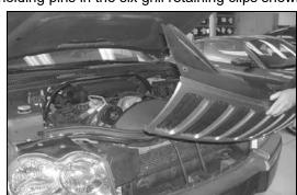
6. Remove the six grill retaining clips from the grill, then tilt the grill froward and remove from the vehicle.
