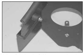
14. Install the bracket/rubber mounted stud assembly onto the heat shield as shown using the provided hardware.
