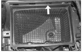
8. Remove the airbox mounting bolt shown.
