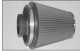
26. Install the filter adapter into the air filter as shown, secure with the provided hose clamp.
