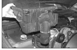
9. Remove the lower airbox from the vehicle as shown.
