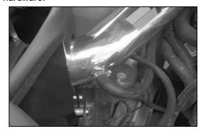
25. Connect the crankcase vent hose onto the K&N® intake tube as shown and secure with the provided hose clamp.
