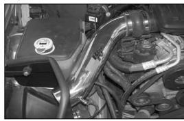
24. Install the K&N® intake tube into the silicone hose at the throttle body and onto the bracket. Secure the tube with the provided hose clamp and hardware.
