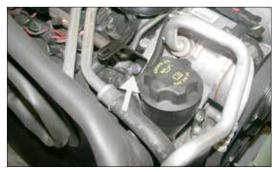
15. Install the tube mounting bracket (010119) onto the A/C compressor using the bolt removed in step #14 as shown.
