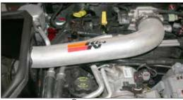
21. Install the K&N<sup>®</sup> intake tube into the throttle body hose and position so the mounting bracket aligns with the tube mounting stand off and then secure with the provided hardware.
