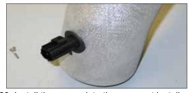
20. Install the sensor into the grommet installed in step #18.
