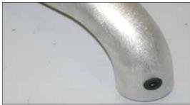
18. Install the provided grommet into the K&N<sup>®</sup> intake tube as shown.
