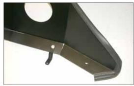
9. Install the "Z" bracket (010120) onto the heat shield with the provided hardware as shown.
