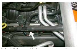
23. Install the provided crank case vent hose onto the factory "TEE" fitting and then onto the  $K\&N^{@}$  intake tube as shown.
