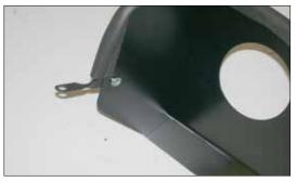
8. Install the twist bracket (070702) onto the heat shield with the provided hardware as shown.
