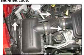
2. Loosen the hose clamp at the intake plenum and the air box mounting nut, and then disconnect the crank case vent hose from the "tee" fitting.
