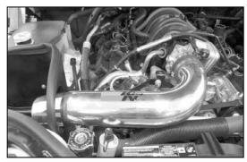
29. Install the K&N<sup>®</sup> intake tube into the silicone hose at the throttle body and onto the tube mounting bracket, then secure with the provided hose clamp and hardware.
