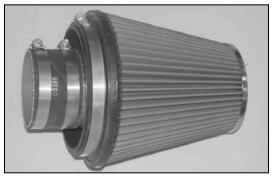
33. Install the silicone (08630) onto the air filter assembly and secure with the provided hose clamp.
