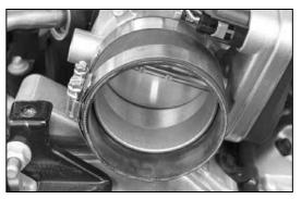
22. Install the silicone hose (08630) onto the throttle body and secure with the hose clamp provided.
