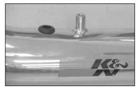
25. Install the provided grommet into the K&N $^{\mbox{\scriptsize \$}}$  intake tube as shown.
