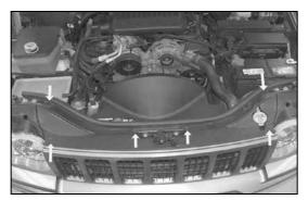
10. Using a small screwdriver, release the center holding pins in the six grill retaining clips shown.
