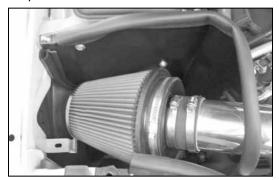
34. Install the air filter assembly onto the K&N<sup>®</sup> intake tube as shown and secure with the provided hose clamp.
