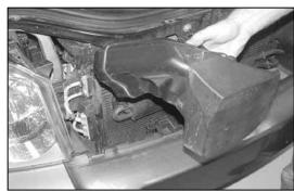
12. Pull the fresh air duct forward to disconnect it from the air box and then remove it from the vehicle.
