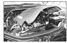
7. Remove the engine cover from the engine.
