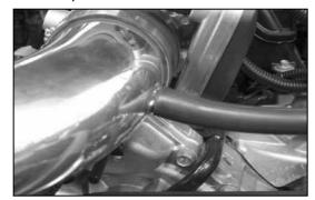
30. Install the provided crank case vent tube onto the valve cover and then onto the  $K\&N^{\otimes}$  intake tube as shown.
