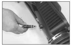
26. Rotate the air temperature sensor counter
