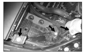
12. Remove the power steering reservoir mounting bolt and the two airbox bracket mounting bolts shown.
