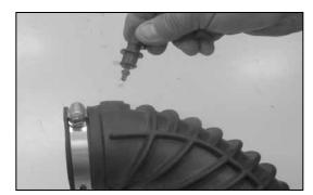
7. Remove the air temperature sensor from the stock intake tube as shown. NOTE: Take care when handling the air temperature sensor as it is very fragile.
