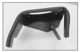
15. Install the supplied bracket (07097) onto the rubber mounted stud as shown. NOTE: Do not completely tighten at this time.
