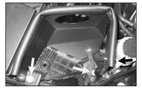
18. Install the heat shield assembly into the engine compartment and secure with the three bolts removed in step #12.
