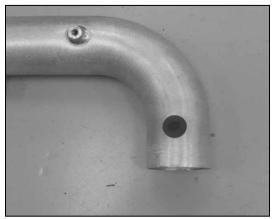
6. Install the supplied grommet into the hole in the K&N $^{\mbox{\tiny 0}}$  intake tube as shown.
