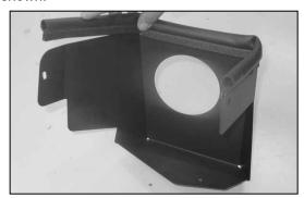
13. Install the supplied edge trim onto the heat shield as shown.
