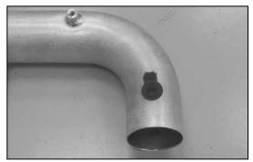
2. Release the locking tab on the air temperature sensor electrical connector and then disconnect the connection.
