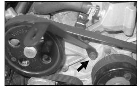
11. Install the supplied tube mounting bracket (26653) onto the engine and secure with the bolt removed in step #10.
