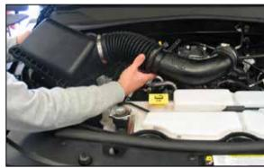
6. Remove the upper airbox and intake tube assembly from the vehicle.
