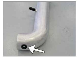
20. Install the provided grommet into the  $K\&N^{\otimes}$  intake tube as shown.
