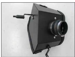
15. Install the bracket/stand-off assembly onto the heat shield using the hardware provided as shown.
