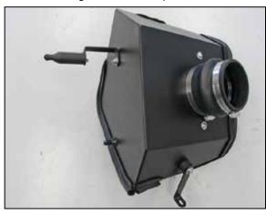
16. Attach the short standoff assembly to the heat shield and secure with the provided hardware as shown.
