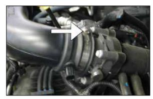
5. Loosen hose clamp at throttle body.
