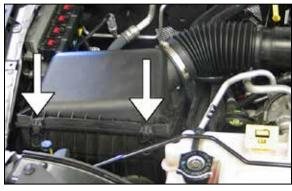
4. Release the two upper airbox retaining clips.
