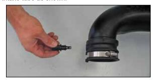
21. Remove inlet air temperature sensor from factory tube as shown.
