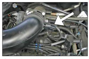
2. Release the red locking tab and then disconnect the inlet air temp sensor electrical connection.
